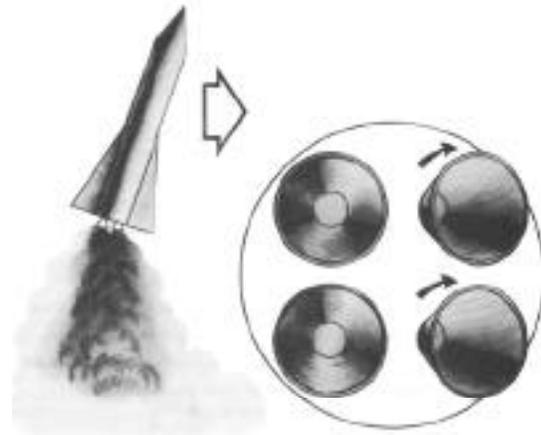
Omniaxis nozzles are capable of moving in any pitch or yaw plane with the use of special load carrying and sealing mechanisms. Since an omniaxis nozzle can provide both pitch and yaw control, only one nozzle is needed, and small secondary thrusters are used for roll control.
