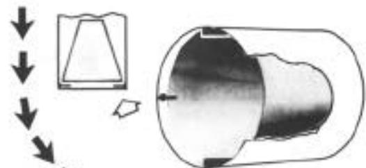
Exhaust gases flow past vane. When activated into flow, gases are diverted by the rudder.
