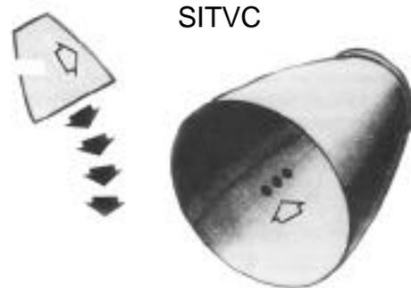
The thrust is deflected by the force of the injected fluid and by the imbalance of pressure created in the nozzle.
