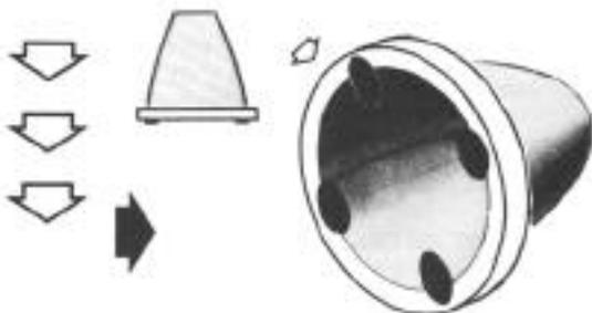
Insertion of the tab creates increased pressure within the exit cone. The diverted force acts to vector the exhaust thrust.
