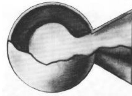
Solid fuel rocket motor with a high mass fraction.
