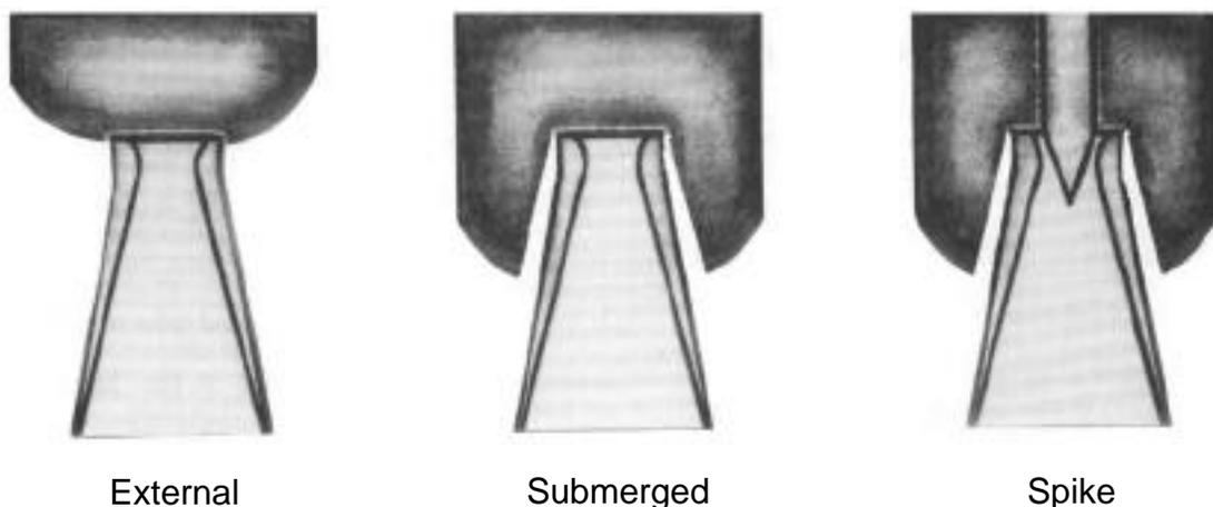
In addition, there are two basic exit cone configurations, conical and contoured. The purpose of contouring the cone is to direct the flow of the exhaust stream so that its force will be concentrated as directly as possible along the longitudinal centerline of the nozzle, thus minimizing flare or divergence of the exhaust stream and concentrating thrust as much as possible.
