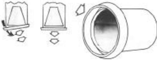
The jet tab system vectors the thrust by insertion of a blunt body (tab) into the supersonic exhaust stream just aft of the nozzle exit plane. Insertion of the tab induces a shock wave and a localized induced pressure area just upstream of the tab, thus producing a side force perpendicular to the axial thrust vector. The thrust vector is controlled by varying the ratio of the jet tab blockage area to the nozzle exit cross sectional area.
