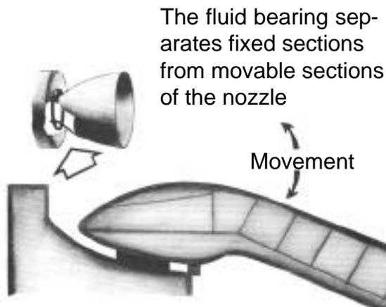
The fluid bearing separates fixed sections from movable sections of the nozzle
