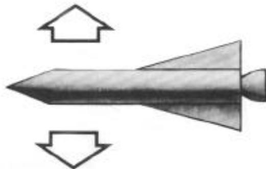
Thrust vector control (TVC) systems can be divided generally into those which change the direction of thrust flow within the fixed nozzle and those which change it with the movable nozzle.
