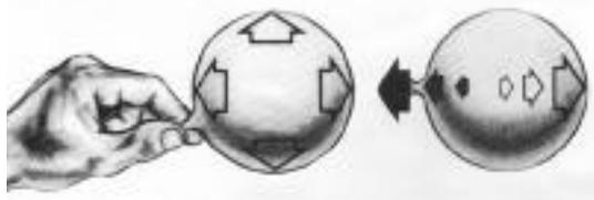
Air pressure equal to all parts of the balloon.
