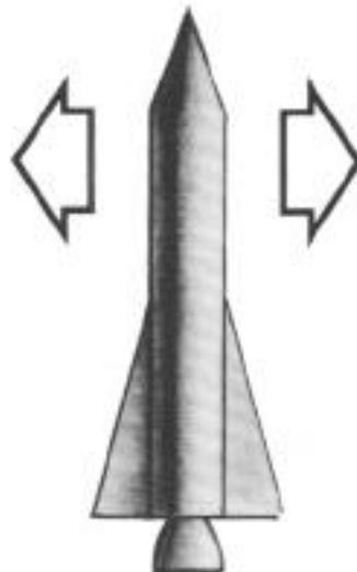
Flight directional control for up or down is referred to as "pitch"
