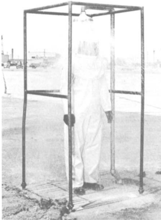
FIGURE 20-4. Plastic safety suit, gloves, boots, and hood used by test personnel in handling hazardous or corrosive liquid propellants. Safety shower, which starts automatically when a person steps onto the platform, washes away splashed or spilled propellant. (Official U.S. Air Force photograph.)
