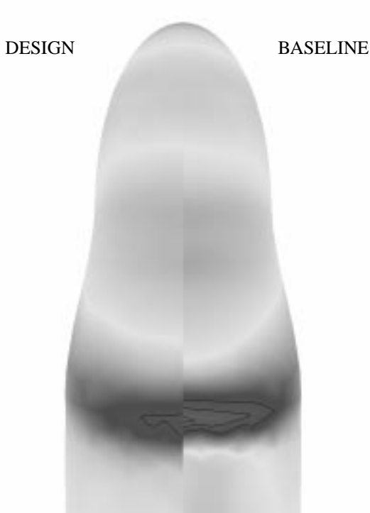
Figure 15. Mach contours in the canopy region for the baseline and design at M=0.75 , C_L=0.48 .
