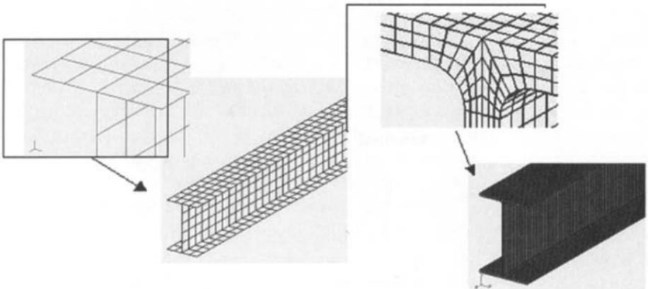
**Fig. 16.12** Plate and brick models for an I-beam.
