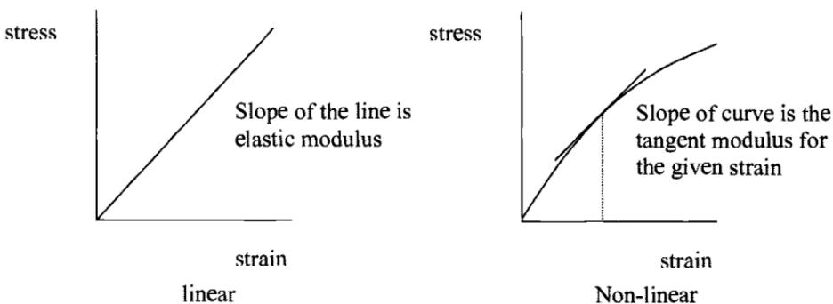
Fig. 16.9 Linear and non-linear material behavior.
