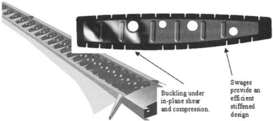
**Fig. 16.2** Design of a structural component.
