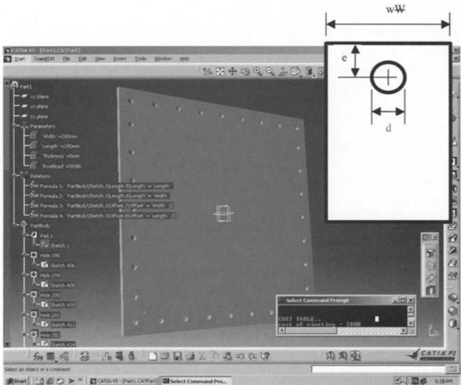
**Fig. 16.1** Design detail in a riveted connection. Ratios  $e/d$  and  $w/d$  affect manufacture, reparability, and durability. Screen shows application of CATIA V5 (Ref. 1).
