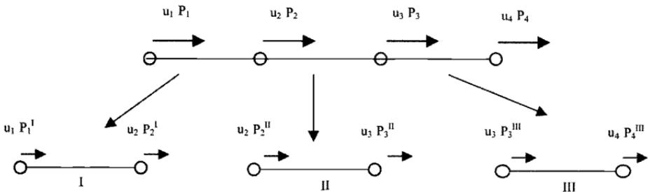
**Fig. 16.7** Discretization into elements.
