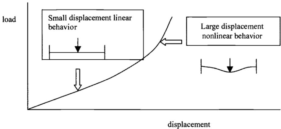
**Fig. 16.10 Linear and non-linear structural behavior. Note: an additional load path is introduced by the deformation of the structure.**
