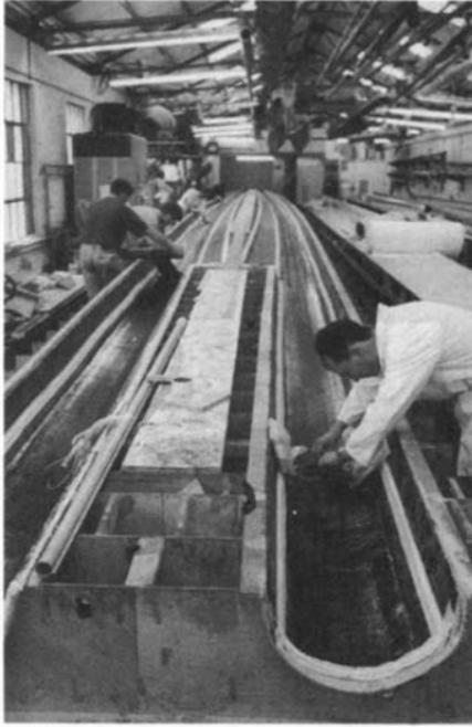
Fig. 15.4 Fiber Bragg grating sensors being embedded in carbon/epoxy composite yacht mast during construction.<sup>10</sup>
