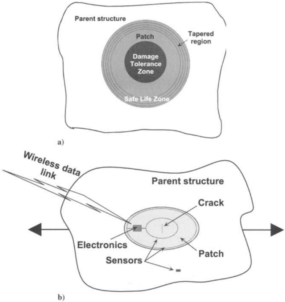
**Fig. 15.2** Schematic diagram of *a*) a generic external bonded repair showing safe-life zone (no disbonding allowed in this zone) and damage-tolerant zone (stable disbonding growth allowed in this zone) and *b*) the smart patch concept.
