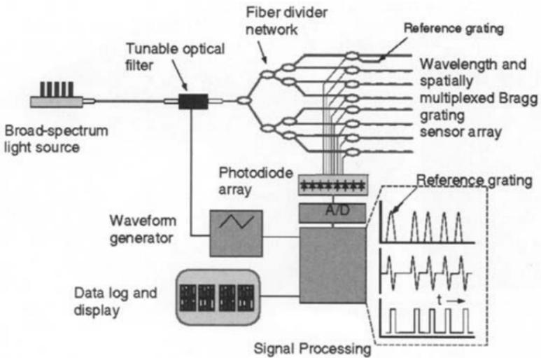
Fig. 15.5 Fiber Bragg grating strain sensor interrogation system architecture used to monitor the fiber Bragg gratings embedded in the carbon/epoxy yacht mast.<sup>10,14</sup>
