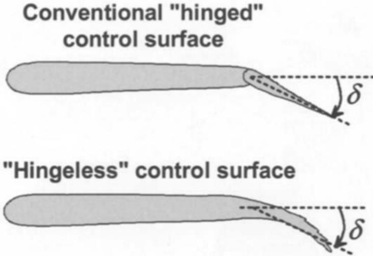
**Fig. 15.12** Schematic diagram of conventional “hinged” control surface and “hingeless” control surface (i.e., morphing structure).
