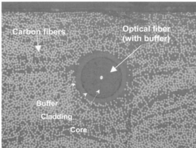
**Fig. 15.3** Micrograph of cross-sectional laminates illustrating a polyimide coated fiber in carbon/epoxy laminate. The carbon fibers have typical fiber diameters of 7  $\mu\text{m}$ , the optical fibers have typical core and cladding diameters of 10  $\mu\text{m}$  and 125  $\mu\text{m}$ , respectively, and the polyimide coating is typically about 12  $\mu\text{m}$  thick.
