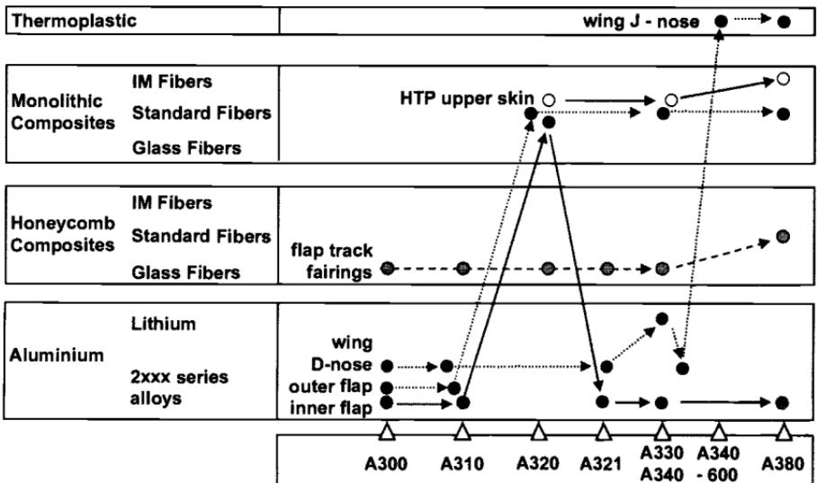
Fig. 12.2 Evolution of Airbus materials selections. Courtesy of Airbus Industries.
