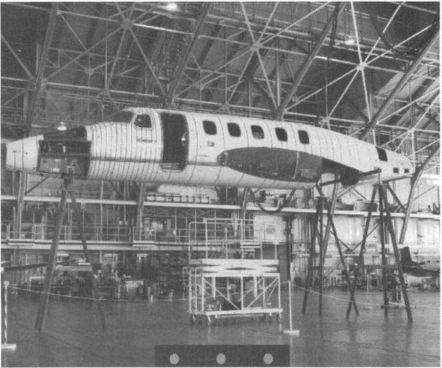
**Fig. 12.3 Premier 1 composite fuselage. Courtesy of the Raytheon Corporation.**
