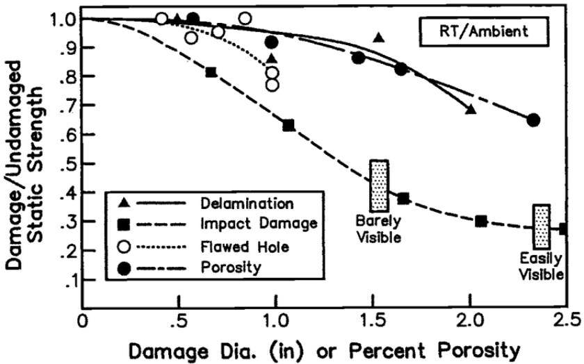
Fig. 12.14 Strength loss associated with impact damage.
