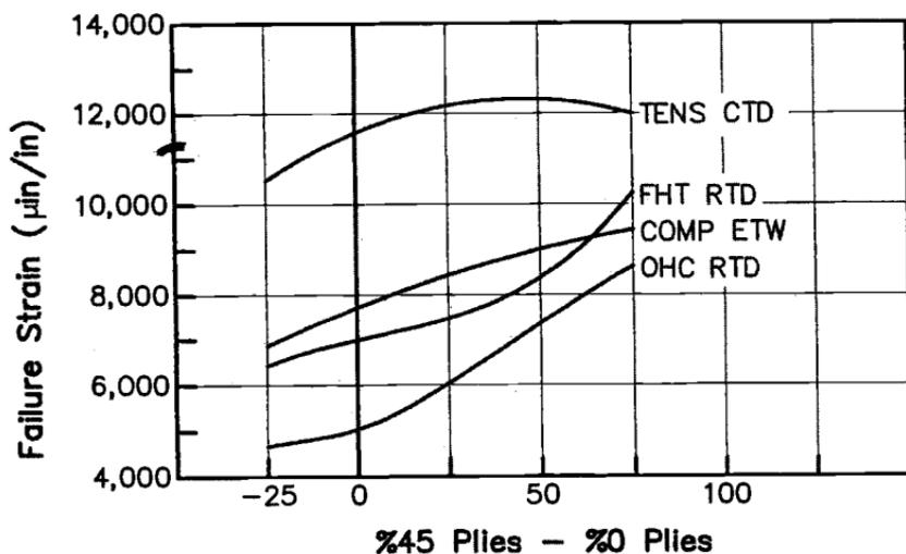
Fig. 12.15 Effect of lay-up on failure strain.
