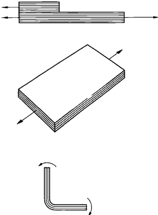
Fig. 12.10 Sources of delamination. Based on Ref. 9.
