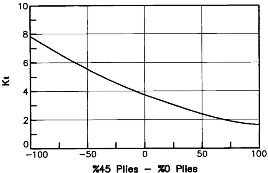
Fig. 12.8 Stress concentration factors in laminates with varying proportions of on- and off-axis plies. Based on Ref. 8.
