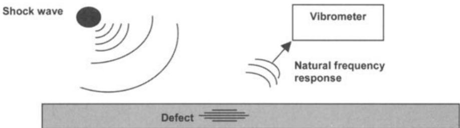
**Fig. 11.16 Schematic of acoustic impact method.**
