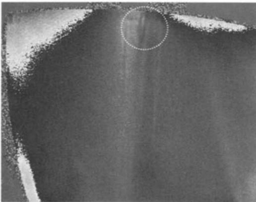
**Fig. 11.13** Shearography image at 8-mm objective of rib to skin junction of composite box structure showing detection of a void. Courtesy of Steinbichler Optotechnik GmbH.
