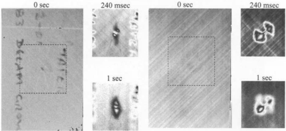
**Fig. 11.12** Flash thermographs of an impact damaged 50 ply carbon/epoxy composites at three stages in the cooling process. Taken from impact surface left and opposite surface right, courtesy of DSTO.
