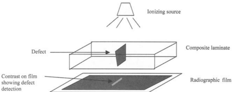
**Fig. 11.7 Schematic diagram of application of X-ray to composite laminate as an NDI method.**
