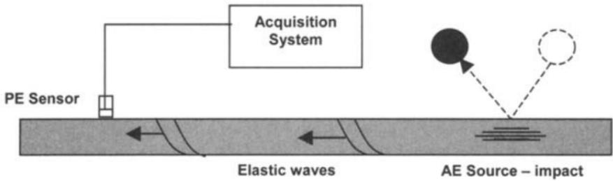
**Fig. 11.14 Schematic of acoustic emission method.**
