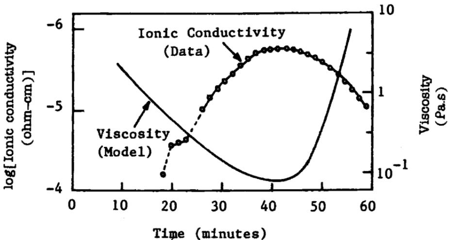
Fig. 11.2 Plot of variation in ionic conductivity and resin viscosity with time during cure of an epoxy resin. Taken from Ref. 11.
