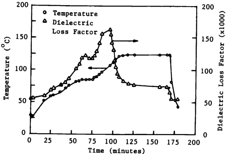
Fig. 11.1 Plot of changes in dielectric loss factor and cure temperature versus time for a glass epoxy pre-preg. Taken from Ref. 11.
