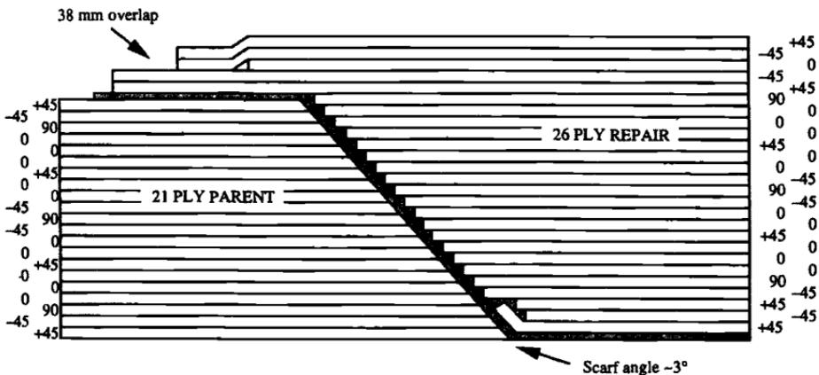
Fig. 10.7 Ply configuration of parent laminate (21 plies) and repair scarf laminate (26 plies). The adhesive (shown shaded) is either FM300 or FM300K structural film adhesive, and the scarf angle is nominally 3°. Taken from Ref. 8.
