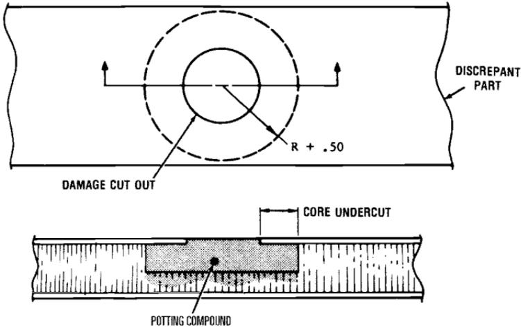
**Fig. 10.2 Potted repair to a damaged honeycomb region.**
