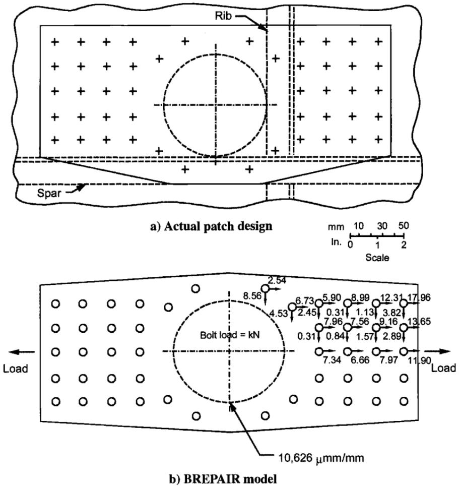
**Fig. 10.12** Schematic illustration of *a*) bolted repair near a spar and rib to a thick laminate, and *b*) predictions of loading at the edge of the repair cut-out and in some of the bolt holes made using the BREPAIR program. Taken from Ref. 17.
