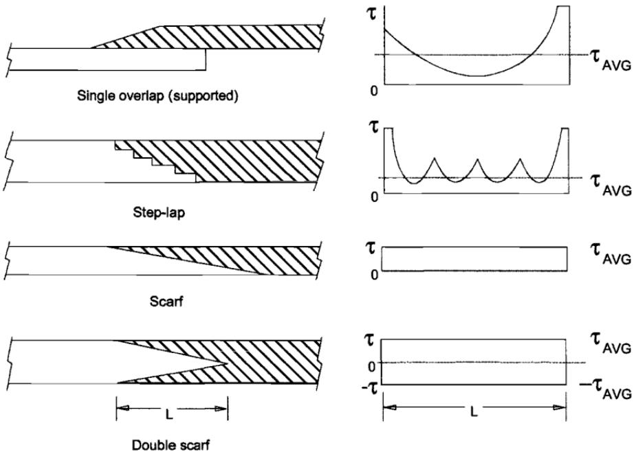
**Fig. 10.4** Main types of joint configuration used for the bonded patch and resulting shear-stress distribution in the adhesive;  $t$  is shear stress and  $\tau_{AVG}$  is the average shear stress.
