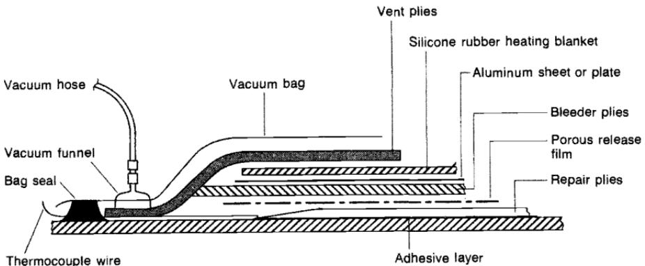
**Fig. 10.10** Vacuum bag and patch arrangement to bond an external patch repair.
