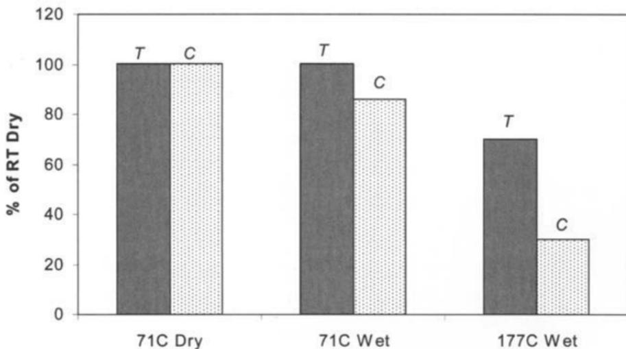
Fig 8.11 Effect of temperature and moisture on tensile  $T$  and compression strength  $C$  of Kevlar 49/epoxy composites in a  $171^{\circ}\text{C}$  cure epoxy resin, compared with value at room temperature. Adapted from Ref. 4.
