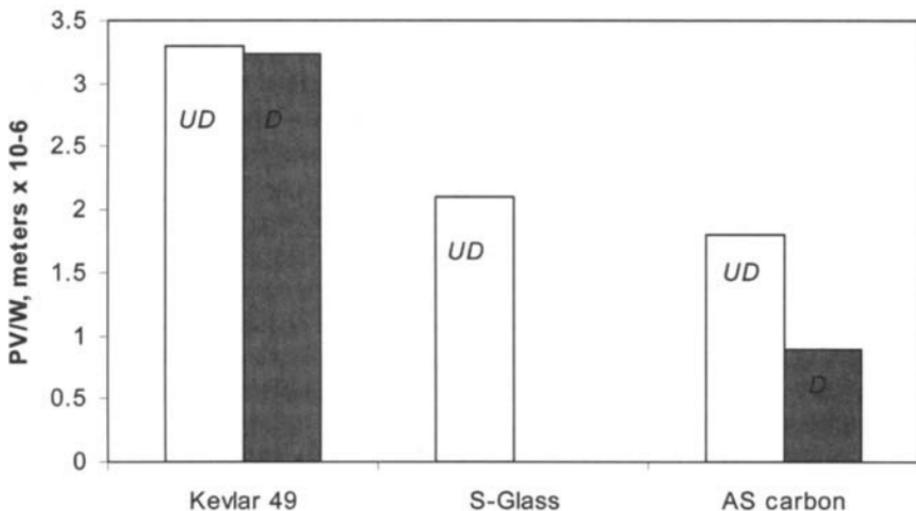
**Fig 8.15 Performance of damaged (D) and undamaged (UD) pressure vessels made in the various composites. Adapted from Ref. 4.**
