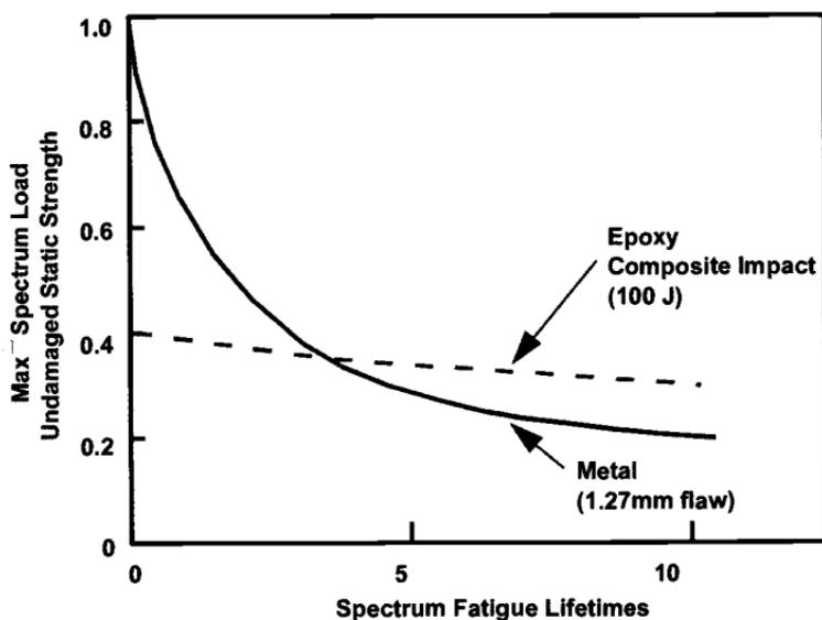
**Fig 8.28** Residual strength as a function of spectrum cycles for 7075 T6 aluminum alloy and carbon/epoxy AS4/3501-6. Adapted from Ref. 14.
