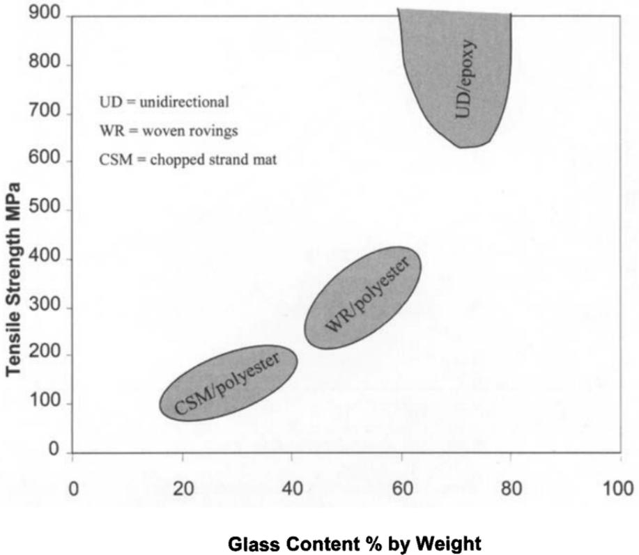
**Fig 8.3** Typical strengths of various types of glass-fiber composites. Adapted from Ref. 1.
