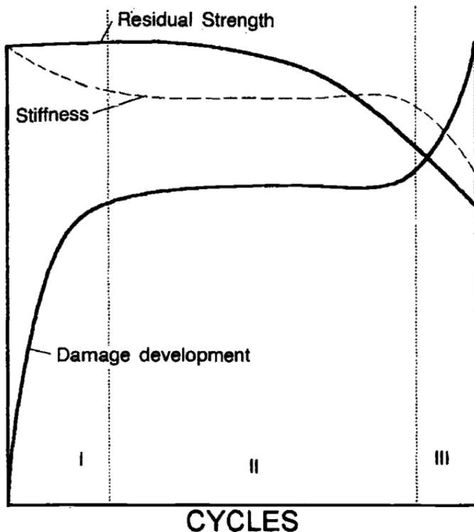
**Fig 8.24** Schematic illustration of the changes in stiffness and residual strength as fatigue damage accumulates. Based on Ref. 2.
