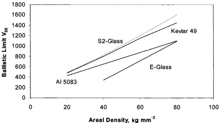
**Fig 8.13** Relative ballistic performance of lightweight armor materials. Adapted from Ref. 4.
