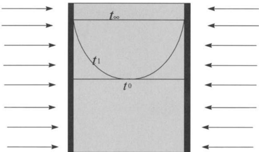
**Fig 8.30** Diffusion of moisture into composite over time.
