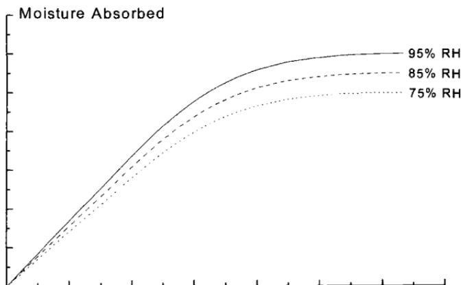
Fig 8.31 Effect of relative humidity on the amount of moisture absorbed with time.
