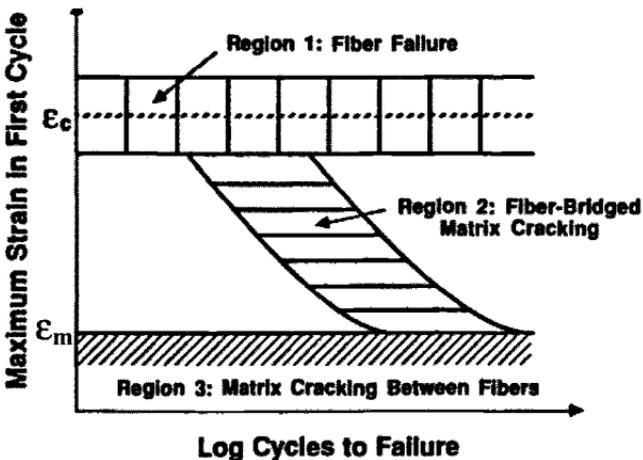
Fig 8.22 Schematic representation of a fatigue-life diagram showing damage zones for a unidirectional carbon-fiber/epoxy composite tested under unidirectional loading. Taken from Ref. 2.
