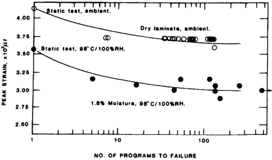
Fig 8.26 Compression residual strength for a 56-ply XAS/914C laminate as a function of spectrum loading representative of that experienced in a fighter wing skin. Behavior under ambient dry and hot/wet is presented. Taken from Ref. 9.
