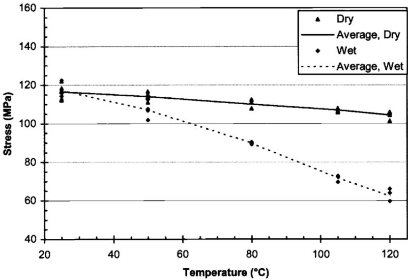
Fig 8.35 Effect of temperature and temperature and moisture of the tensile strength of  $\pm 45^\circ$  laminates of AS4/3501-6. Taken from Ref. 17.
