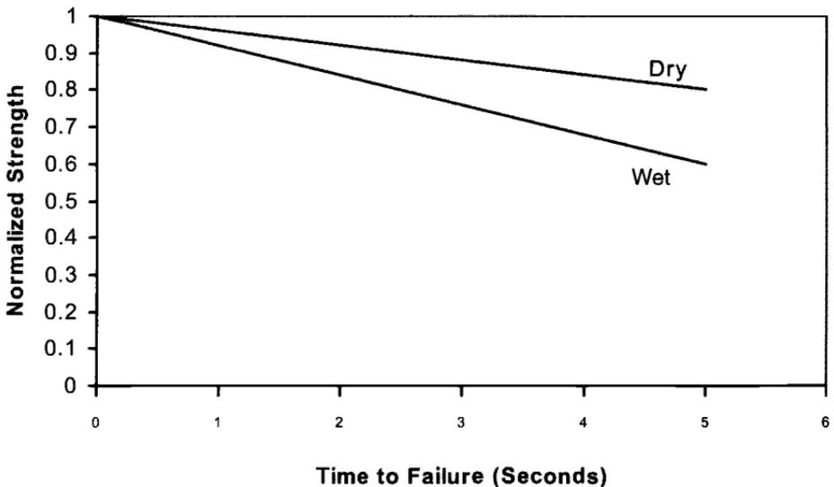
Fig 8.7 Stress rupture strength of E-glass fibers in air and water. Adapted from Ref. 1.
