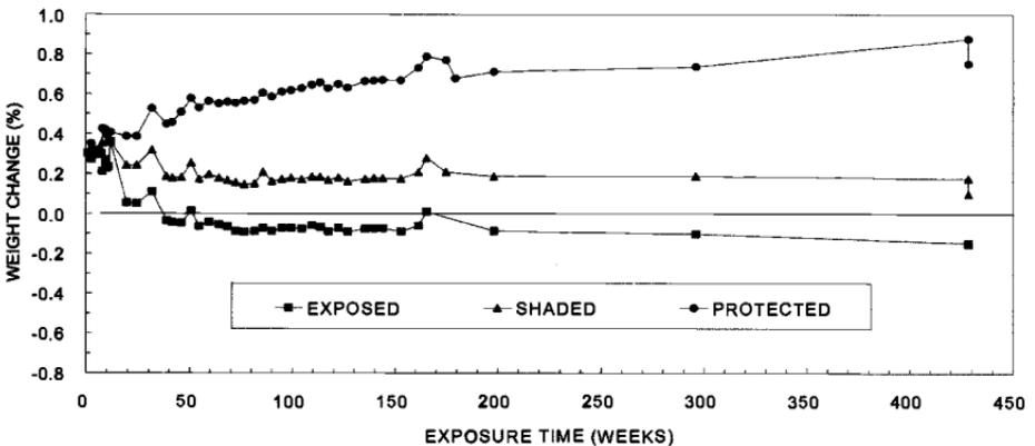
**Fig 8.33** Weight changes for unpainted composite coupons (20-ply AS4/3501-6) exposed at Butterworth Air Force Base in Malaysia. Taken from Ref.16.
