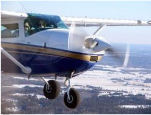
1967 Model Cessna 182K in flight showing after-market vortex generators on the wing leading edge
