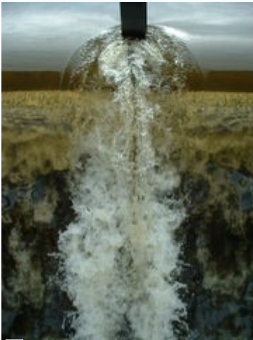
Turbulent flow around an obstacle; the flow further upstream is laminar
