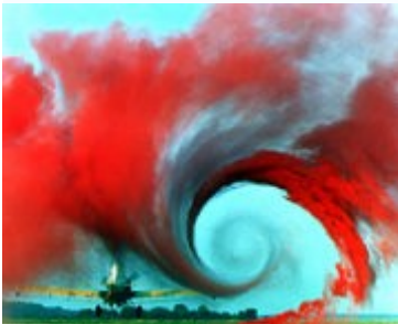
Turbulence in the tip vortex from an airplane wing
