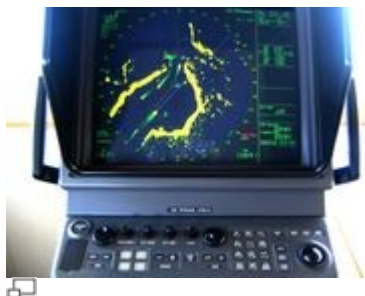
Surface search radar display commonly found on ships
