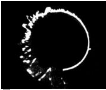
The effect of chaff on the display of a Giant Wurzberg
