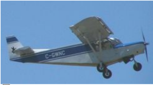
A Zenair CH 701 STOL showing its fixed, full span leading edge slots in flight
