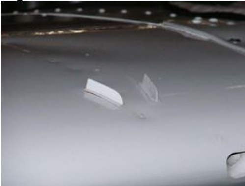
After-market Micro Dynamics vortex generators mounted on the wing of a Cessna 182K
