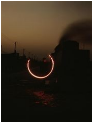
A IHB brakeman uses a fusee to demonstrate a hand signal indicating "stop".
