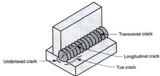
Various forms of Welding Cracks
