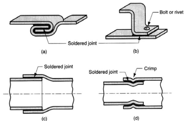
(a) Flat lock seam (b) Bolted or riveted joint (c) Copper pipe fitting (d) Crimping of cylindrical lap joint.
