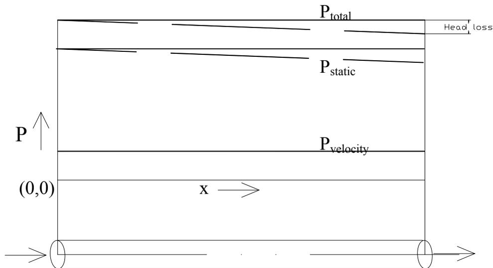
**Fig. 6.2.** Application of Bernoulli equation to pipe flow
