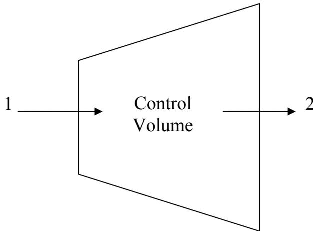
Fig. 6.1. Steady fluid flow through a duct
