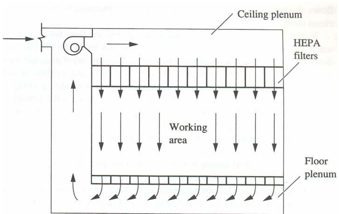
**Fig.39.12(a):** Downward unidirectional flow
