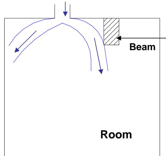
**Fig.39.1(b):** Deflection of a cool air jet
