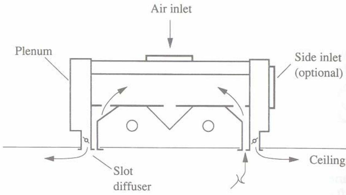
**Fig.39.8:** Light troffer-diffuser slot
