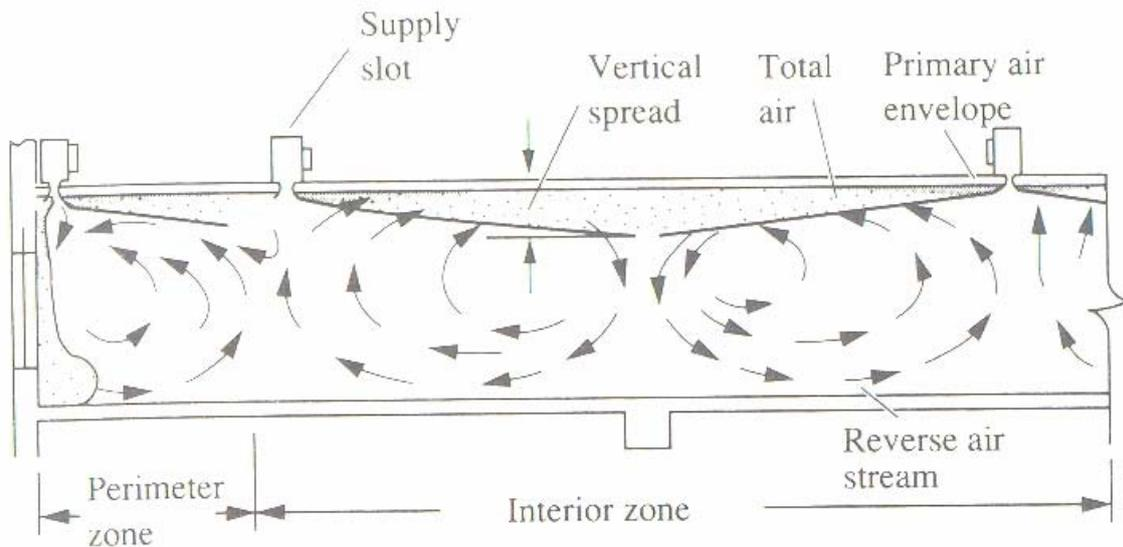
**Fig.39.11:** Airflow pattern for cooling using slot diffusers
