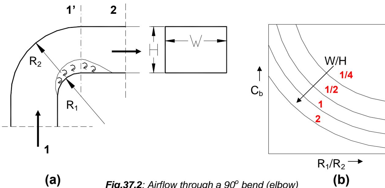
The cross-section of the elbow could be circular or rectangular. Weisbach proposed that the dynamic pressure loss in an elbow is due to the sudden expansion from the *vena contracta* region (1') to full cross-section 2 as shown in Fig.37.2(a). The dynamic pressure drop due to the elbow or  $90^\circ$  turn is found to be a function of the aspect ratio ( $W/H$ ), inner and outer radii of the turn ( $R_1$  and  $R_2$ ) and the velocity pressure  $\rho V^2/2$ , i.e.,
