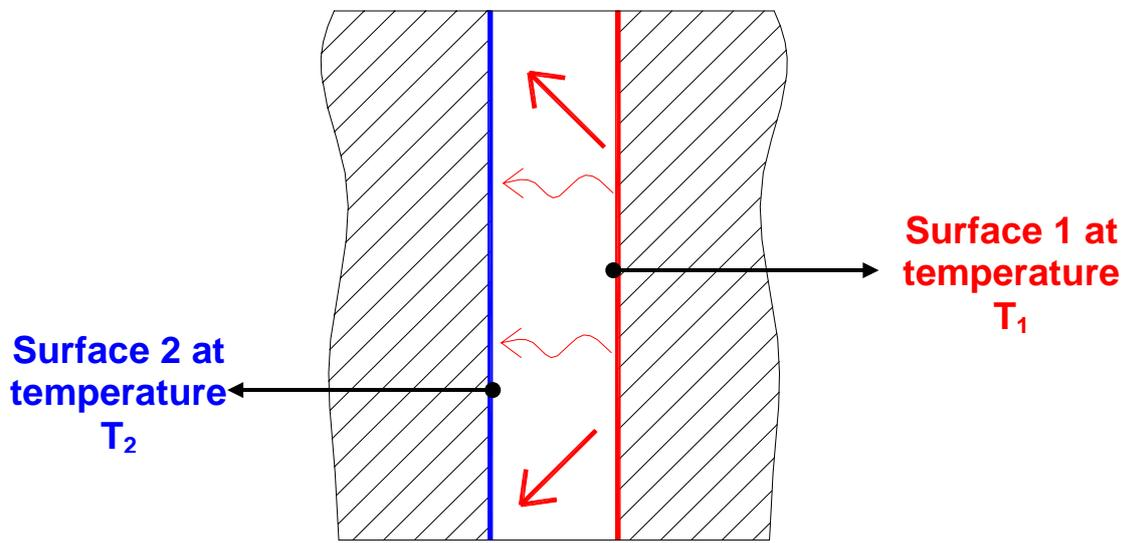
**Fig.34.3:** Heat transfer through an air space in the wall
