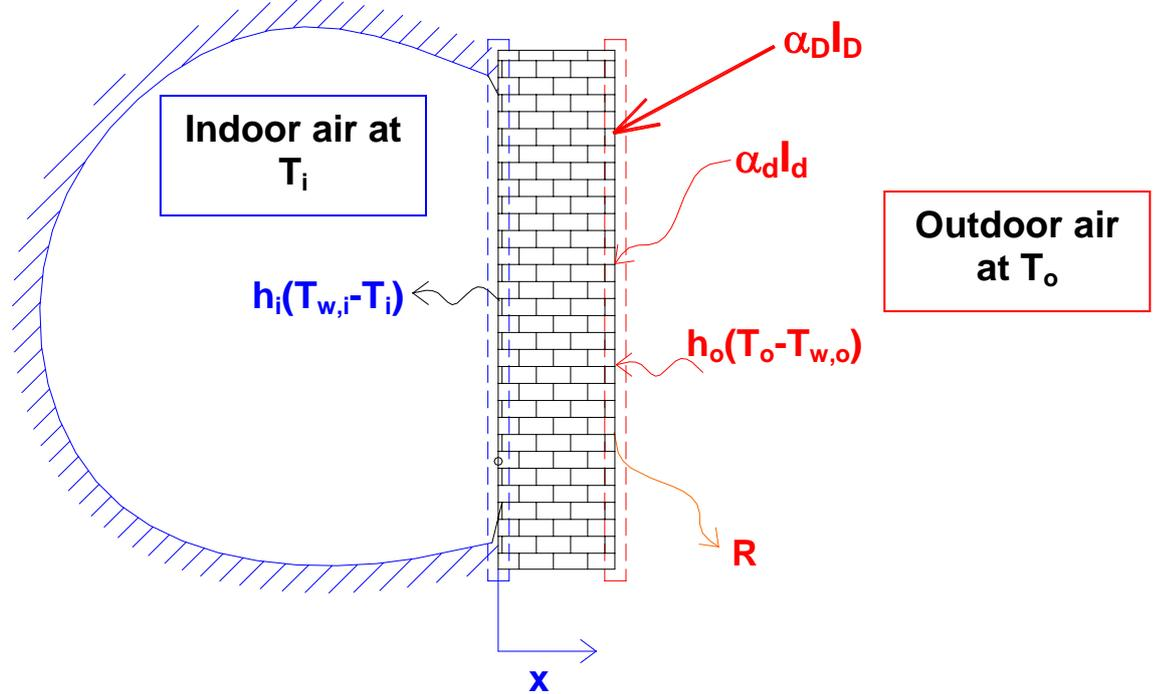
**Fig.34.4.** Unsteady heat transfer through a building wall
