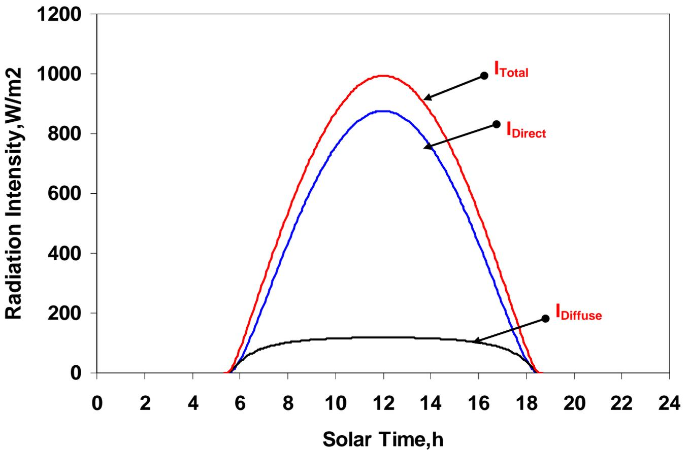
**Fig.34.5:** Variation of direct, diffuse and total solar radiation on a horizontal surface with time under clear sky conditions
