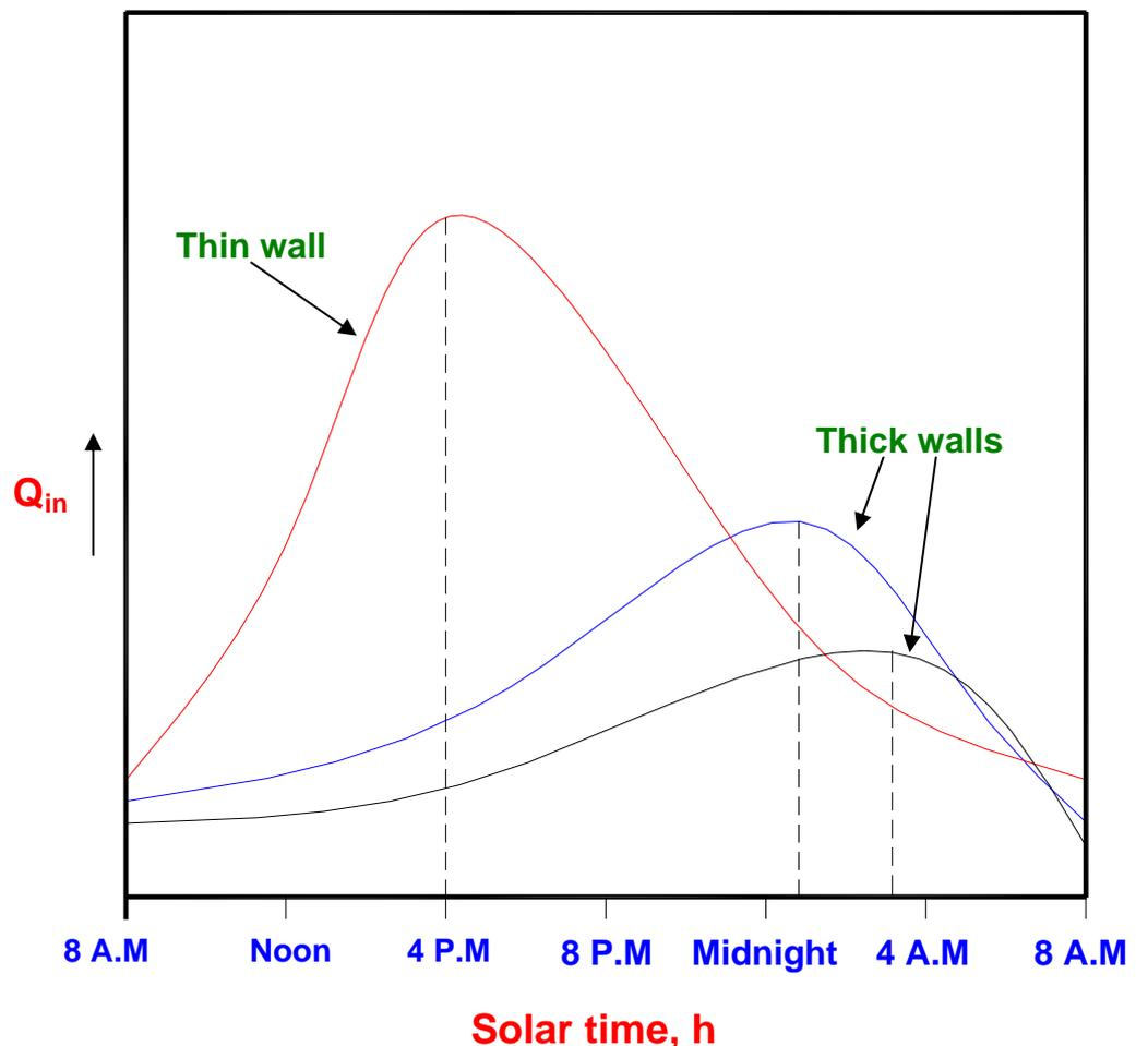
**Fig.34.7:** Variation of heat transfer rate with time for thick and thin walled buildings
