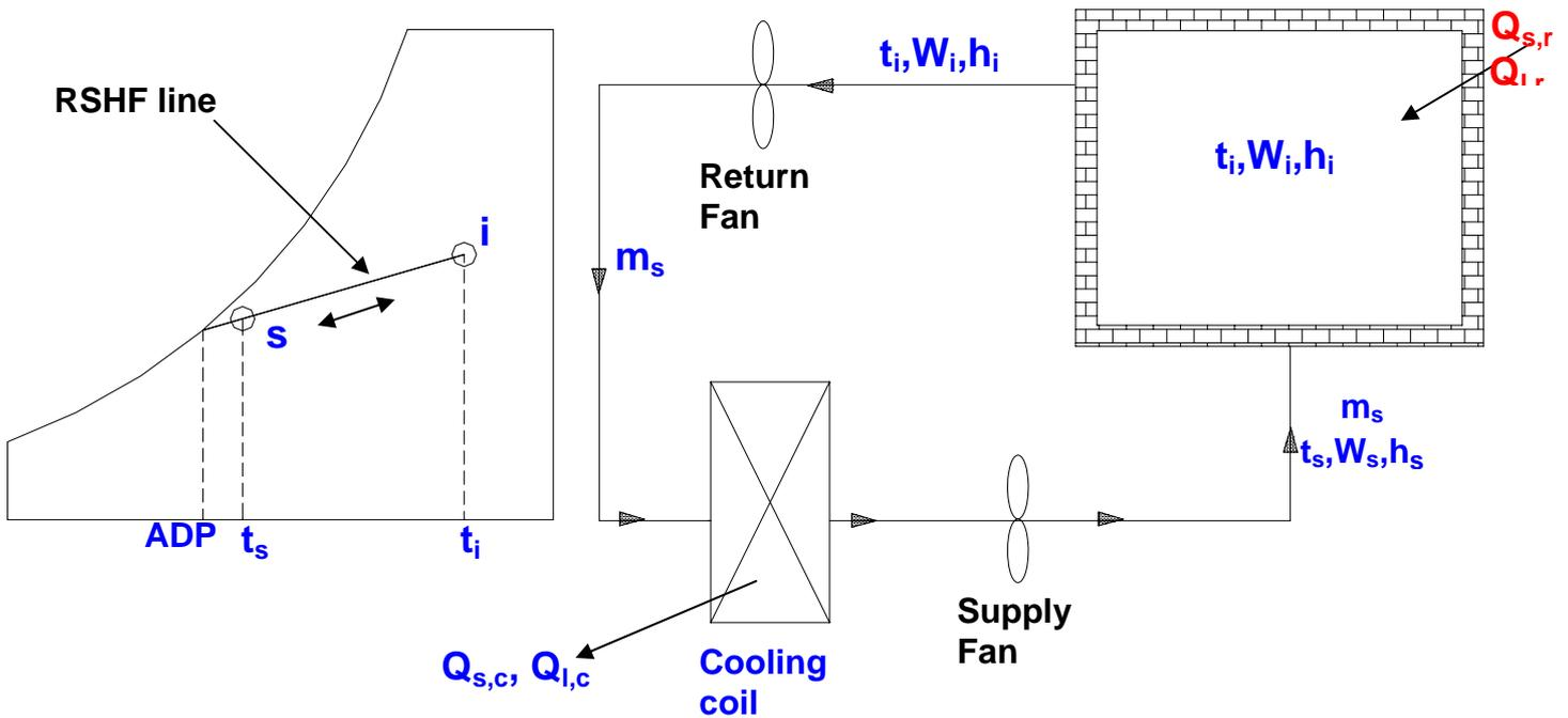
**Fig.30.1:** A simple, 100% re-circulation type air conditioning system
