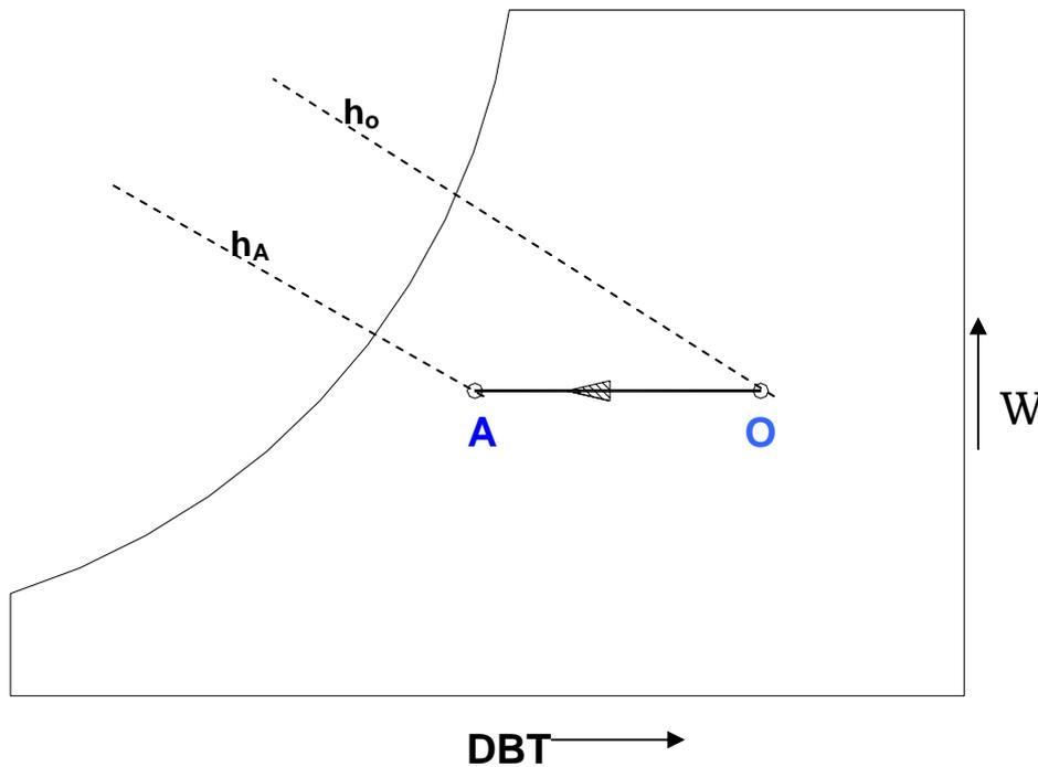
**Fig.28.1:** Sensible cooling process O-A on psychrometric chart
