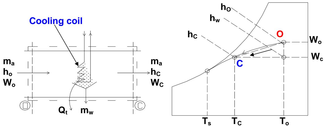
**Fig.28.3:** Cooling and dehumidification process (O-C)
