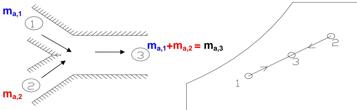
**Fig.28.8.** Mixing of two air streams without condensation
