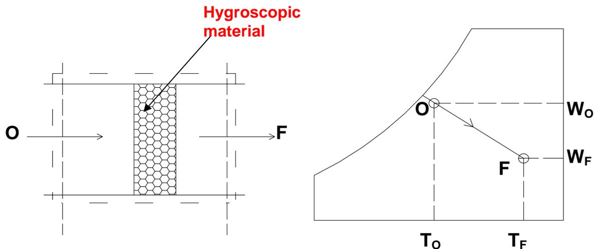
**Fig.28.7.** Chemical de-humidification process
