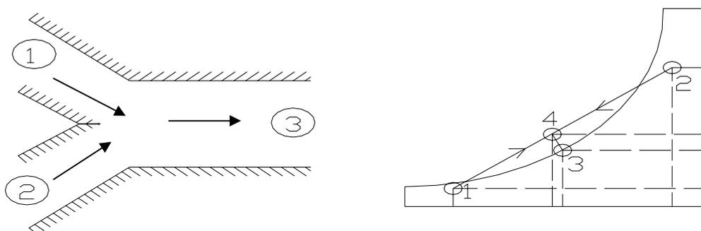
**Fig.28.9.** Mixing of two air streams with condensation
