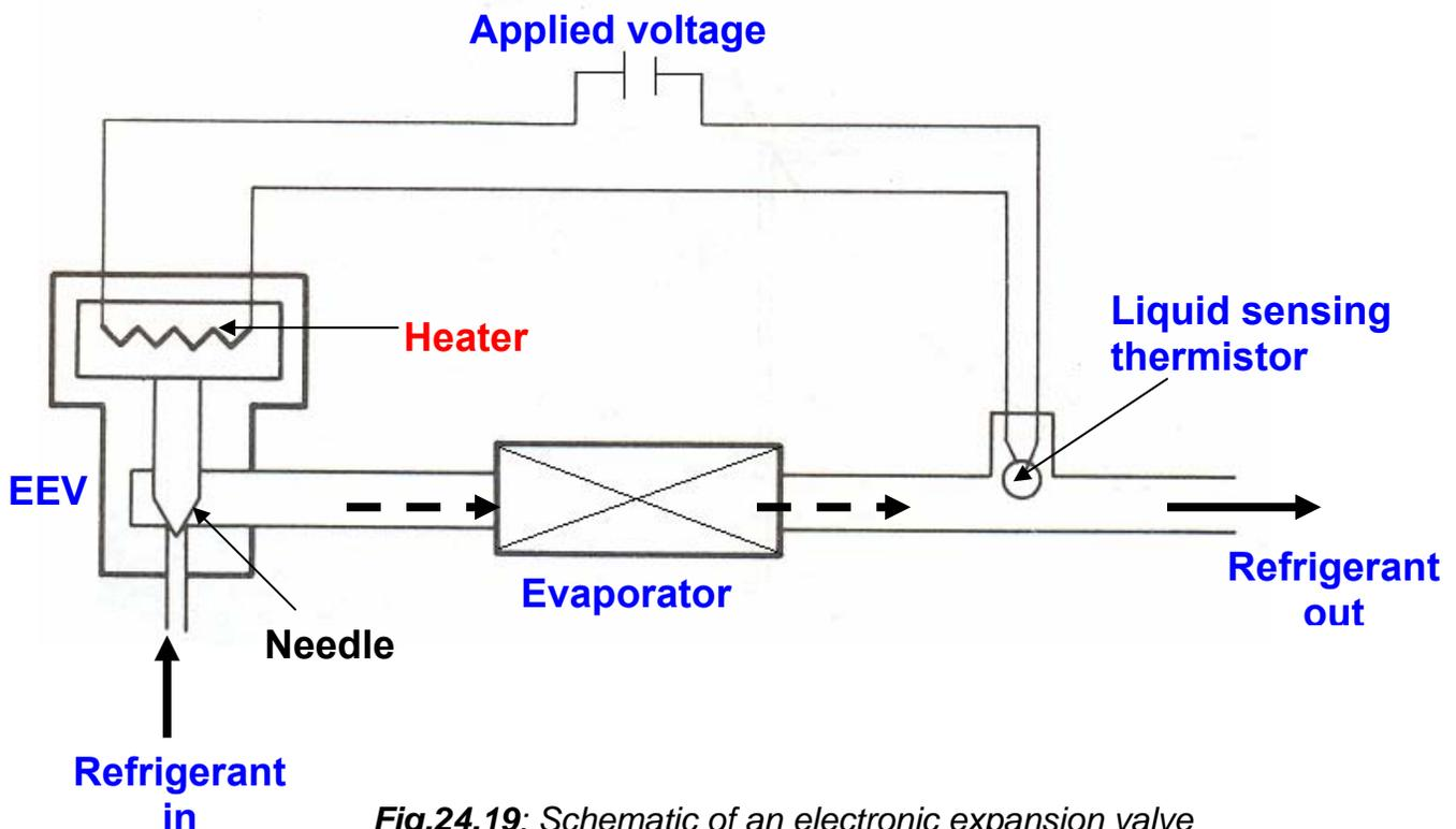
Fig.24.19: Schematic of an electronic expansion valve
