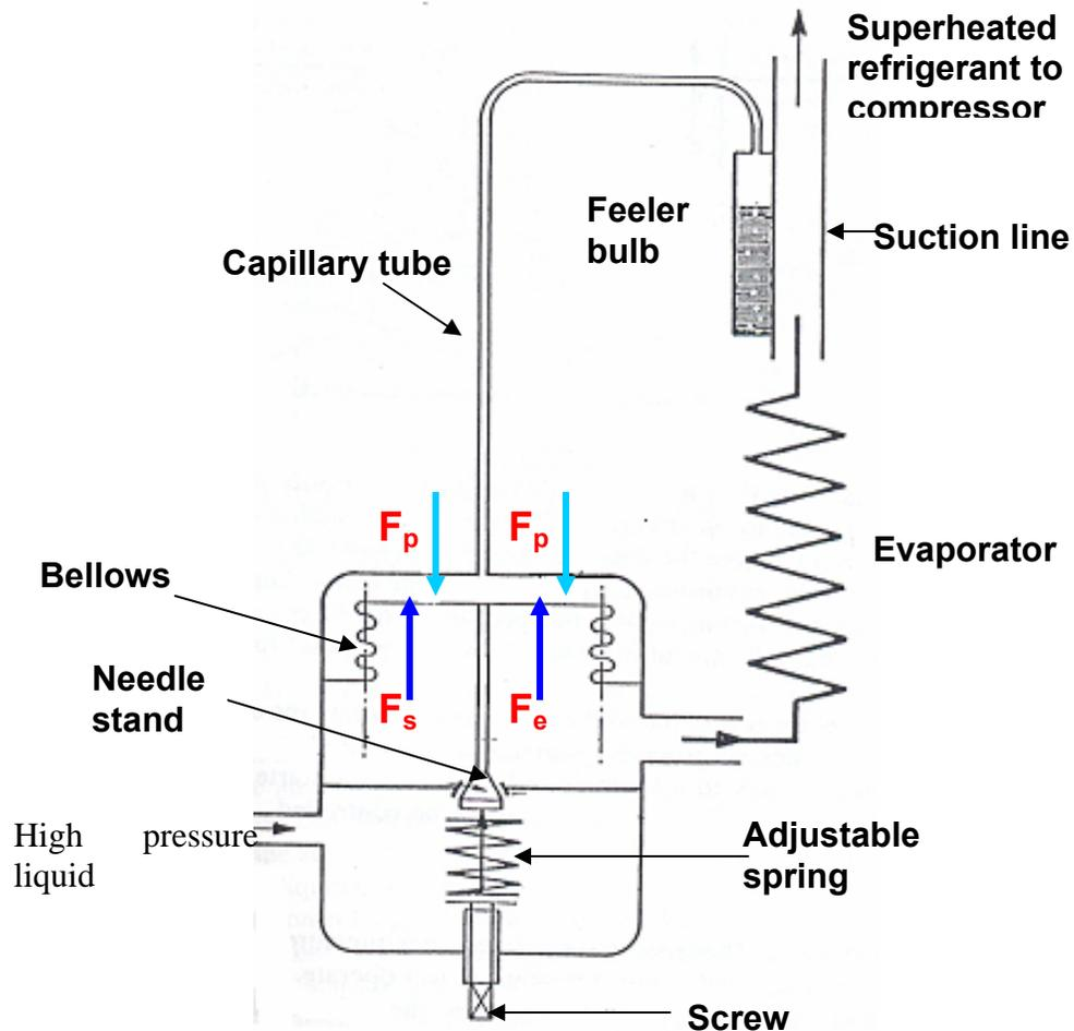
**Fig.24.13:** Schematic of a Thermostatic Expansion Valve (TEV)
