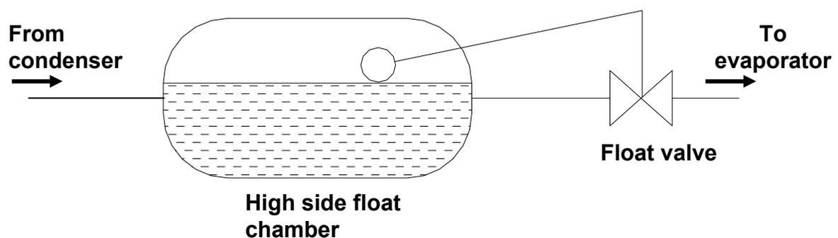
**Fig.24.18:** Schematic of a high-side float valve
