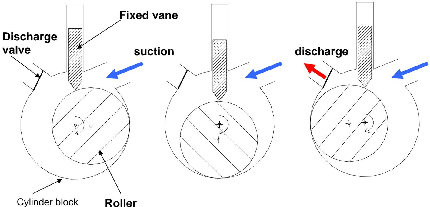
**Fig.20.1:** Working principle of a rolling piston type compressor
