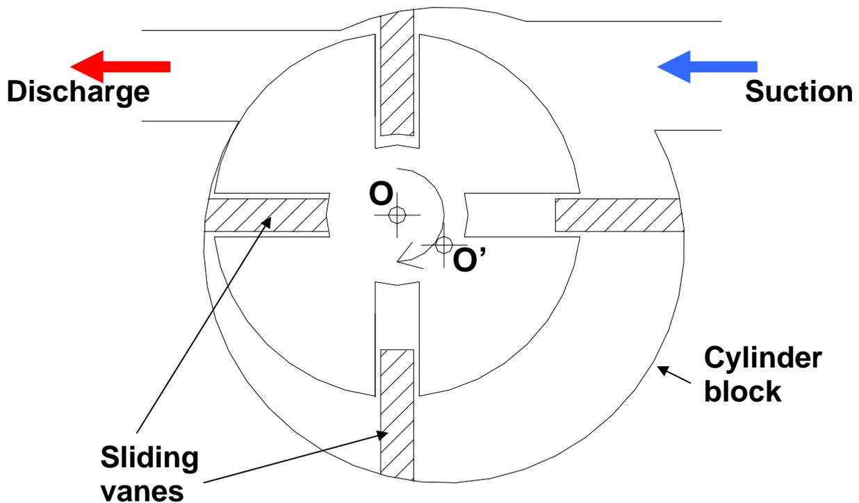
**Fig.20.2:** Working principle of a multiple vane, rotary compressor
