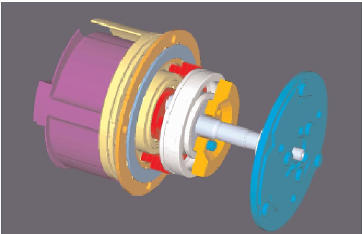
The graphic shown above shows a side view of the interior components of the scroll compressor.
