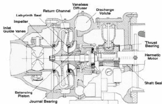
Fig. 2.7 Cut-view of a two-stage, semi-hermetic centrifugal compressor.
