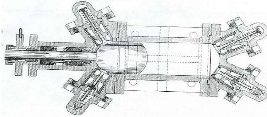
*Fig.2.1. Schematic of Linde's horizontal, double acting compressor*
