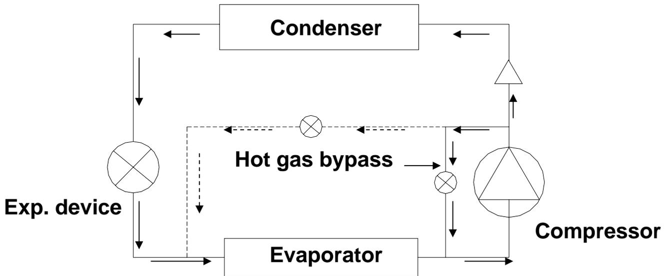
**Fig.19.12:** A vapour compression refrigeration system with hot gas bypass arrangement
