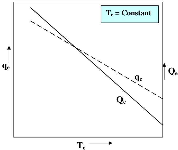
**Fig.19.7.** Effect of condenser temperature on refrigeration effect and refrigeration capacity
