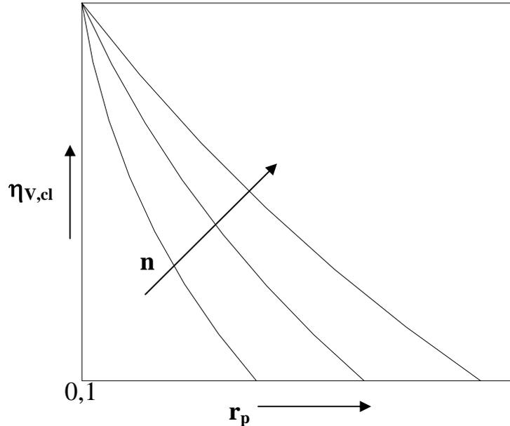
**Fig.18.5.** Effect of pressure ratio ( $r_p$ ) and index of compression ( $n$ ) on clearance volumetric efficiency ( $\eta_{v,cl}$ )
