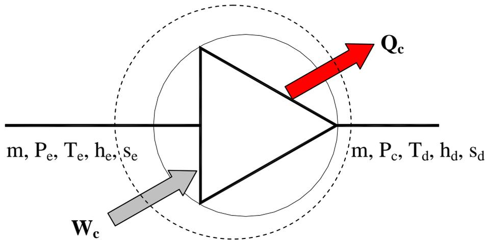
**Fig.18.3.** Energy balance across a steady flow compressor
