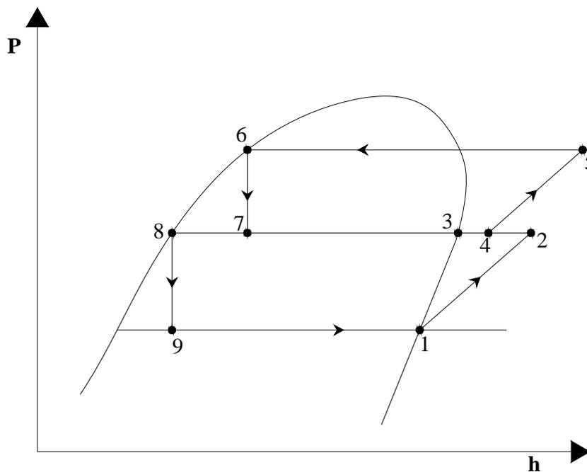
**Fig.12.8:** A two-stage compression system with flash tank for flash gas removal only
