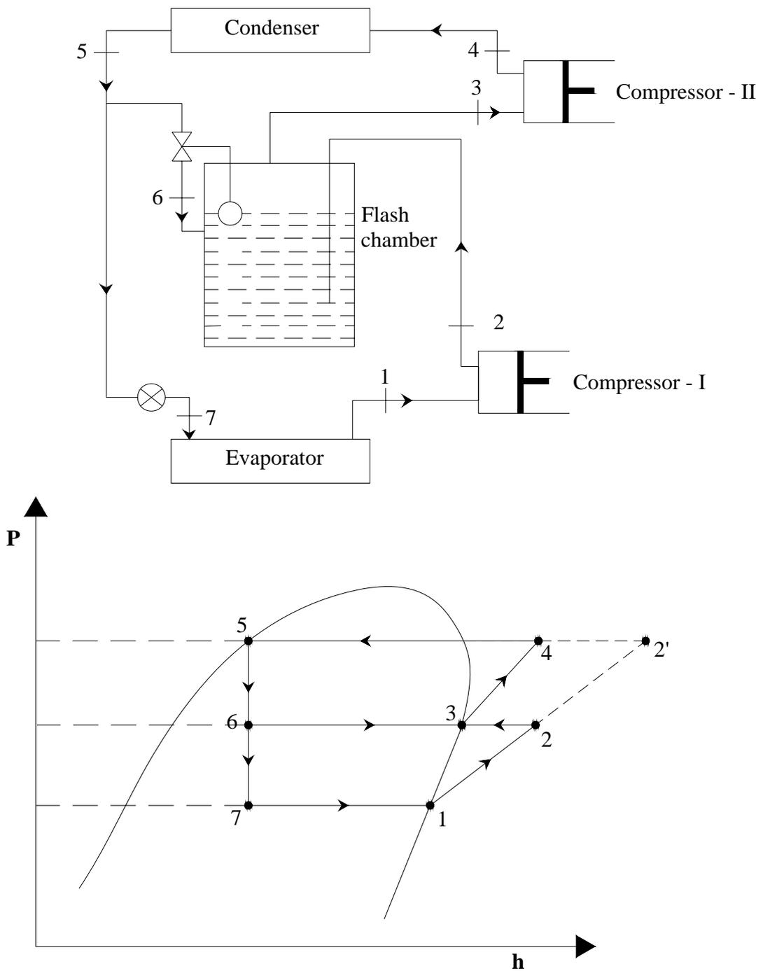
**Fig.12.9:** A two-stage compression system with the flash tank used for intercooling only
