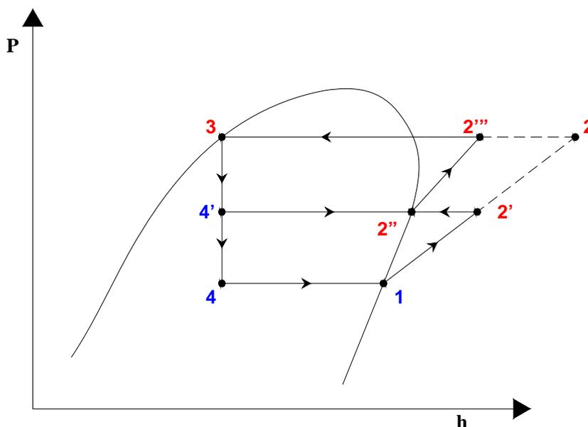
Required refrigerant mass flow rate through evaporator and 1<sup>st</sup> stage compressor ( $m_{r,1}$ ) is same as that of single stage system, i.e.,
