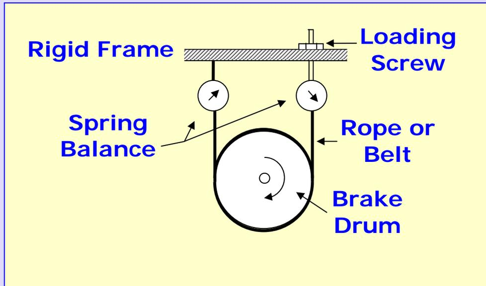
**Figure 60 Schematic of a brake drum dynamometer**
