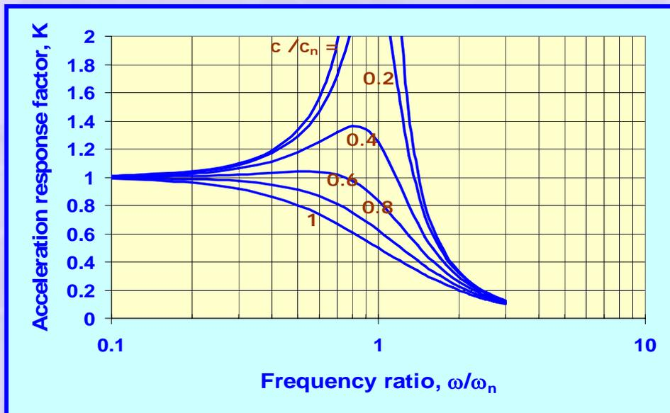
**Figure 57 Acceleration response of a second order system**
