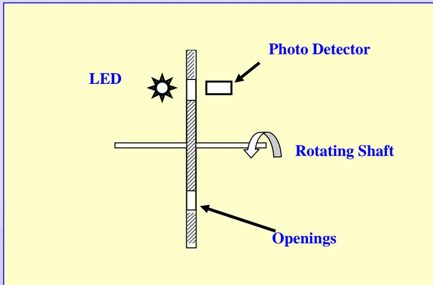
**Figure 66 Optical rpm measurement**
