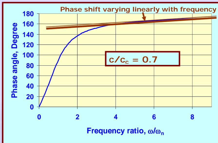
**Figure 56 Phase lag of a system with damping ratio of 0.7**
