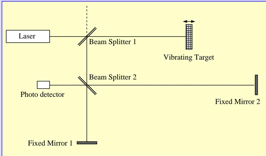
**Figure 58 Schematic to explain the working principle of a Laser Doppler Vibrometer**
