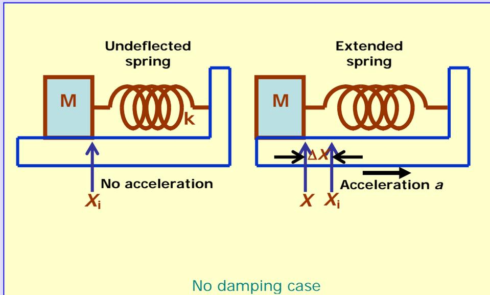
**Figure 50 Spring mass system under the influence of an external force**
