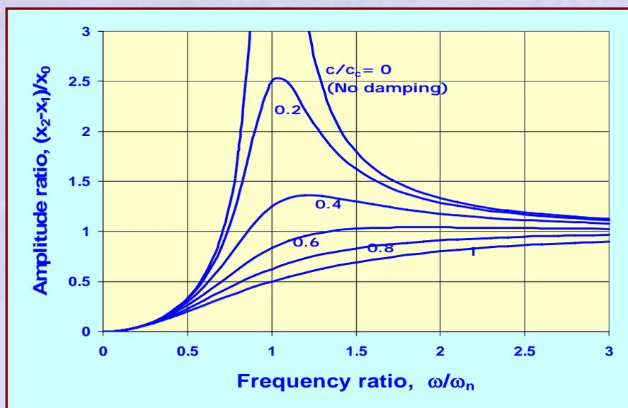
**Figure 52 Steady state response of a second order system to periodic input**
