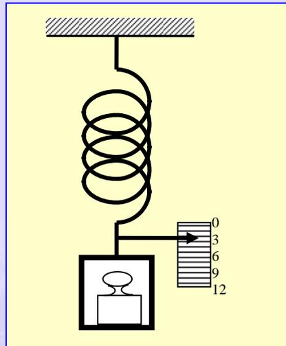
**Figure 48 Schematic of a spring balance**
