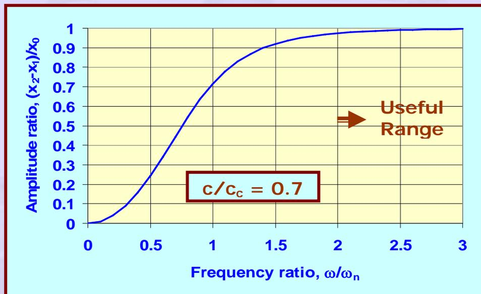
Figure 55 Amplitude response of a system with damping ratio of 0.7
