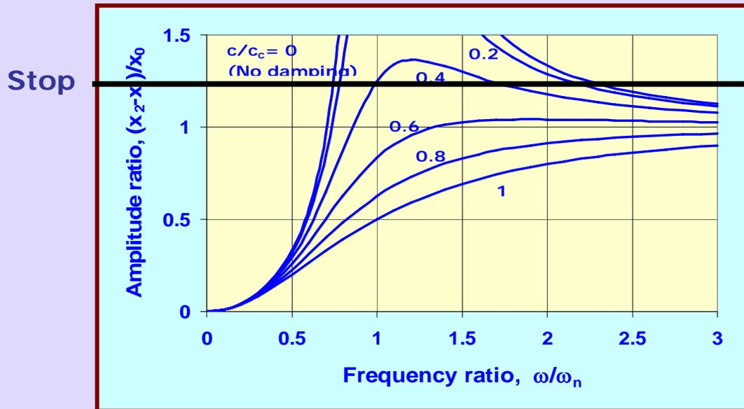
**Figure 53 Steady state response of a second order system to periodic input with amplitude limiting stops**
