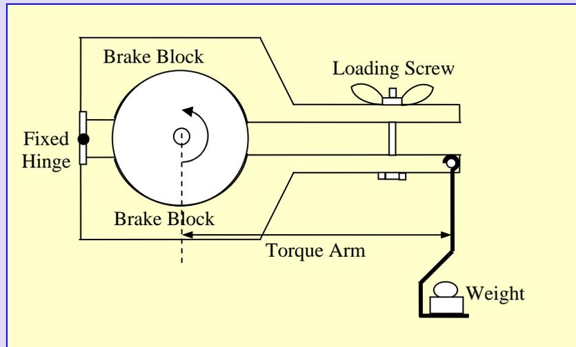
**Figure 61 An alternate method of measuring torque with a Prony brake**
