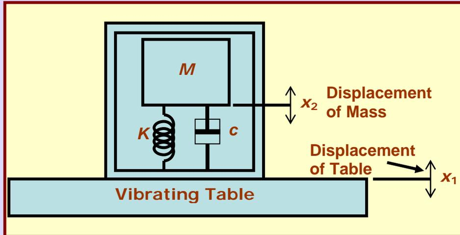
**Figure 51 Schematic of a vibration or acceleration measuring system**
