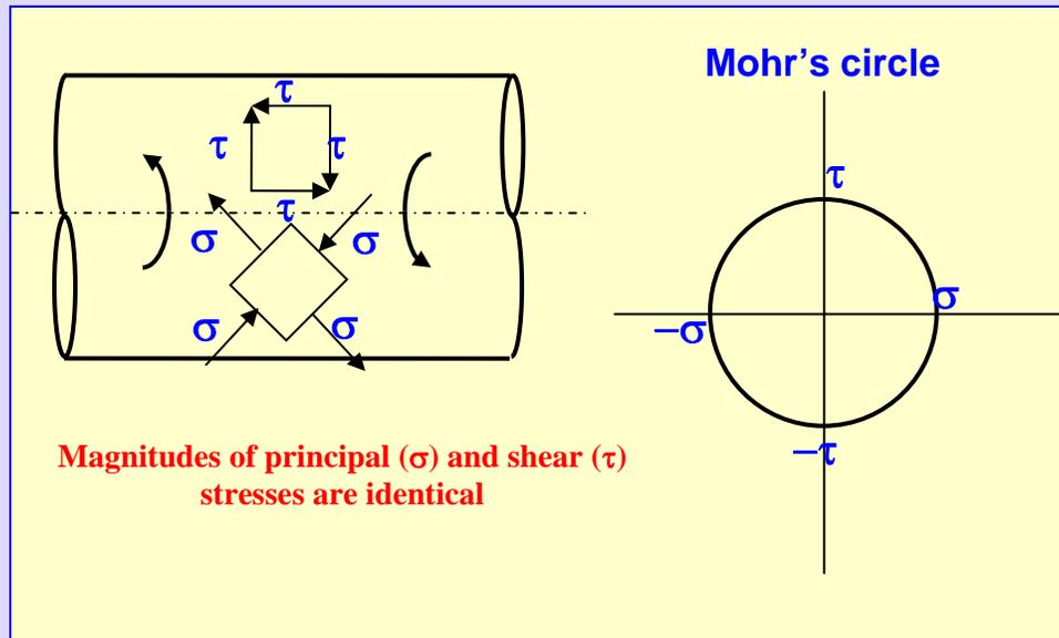
**Figure 63 Stresses on the surface of a shaft in torsion**
