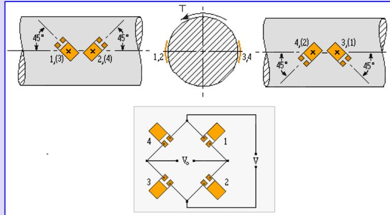
**Figure 64 Strain gages for shear measurement**
