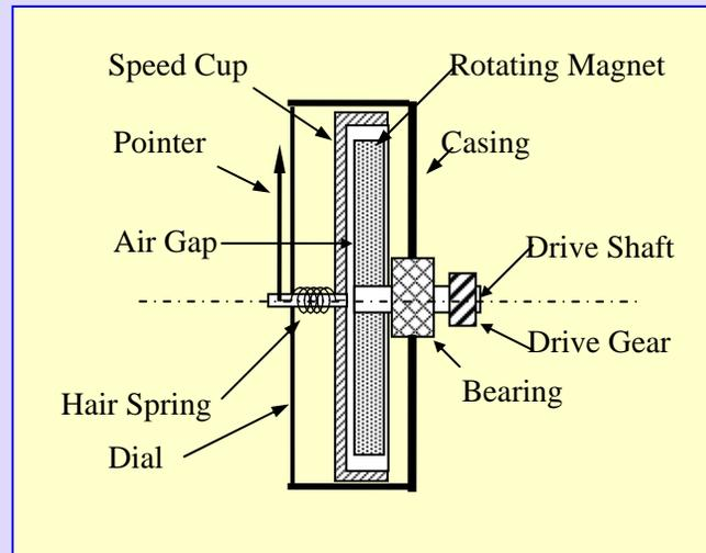
**Figure 65 Speedometer or tachometer**
