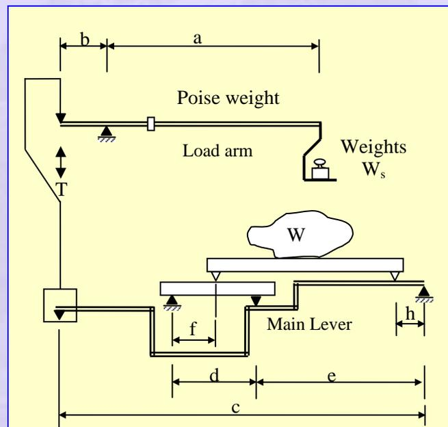
**Figure 47 Sectional skeletal view of a platform balance**
