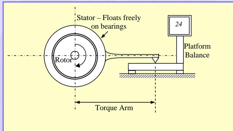
**Figure 62 Electric generator used as a dynamometer**
