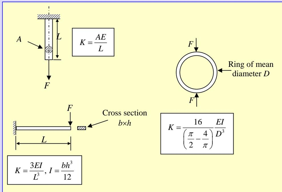
**Figure 49 Several configurations for measuring force with the appropriate spring constants: (a) Rod in tension or compression (b) Cantilever beam (c) Thin ring**
