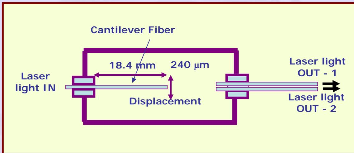
**Figure 59 Schematic of a fiber optic accelerometer**
