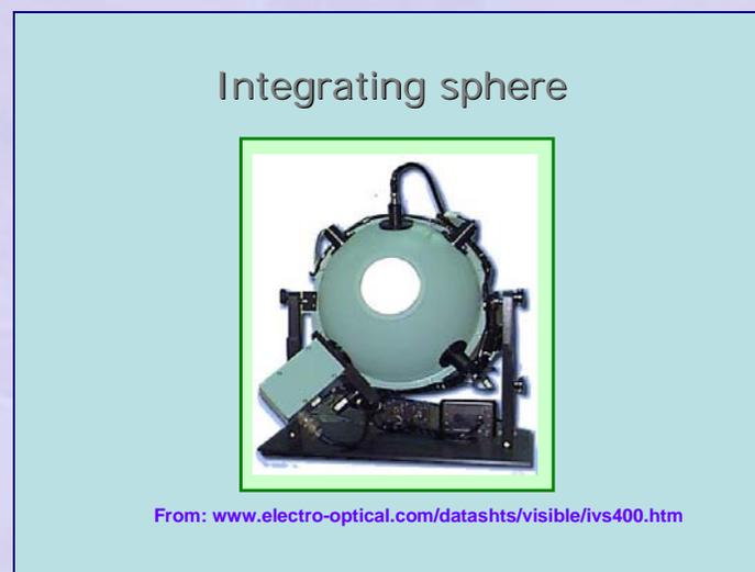
**Figure 27 Photograph of an integrating sphere**
