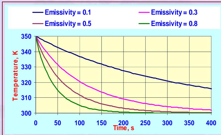
**Figure 32 Cooling history of a heated object in vacuum**
