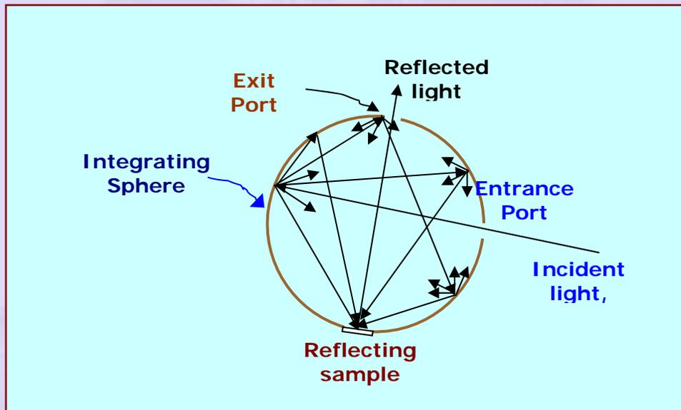
**Figure 29 Integrating sphere arranged for measurement of hemispherical directional reflectivity**
