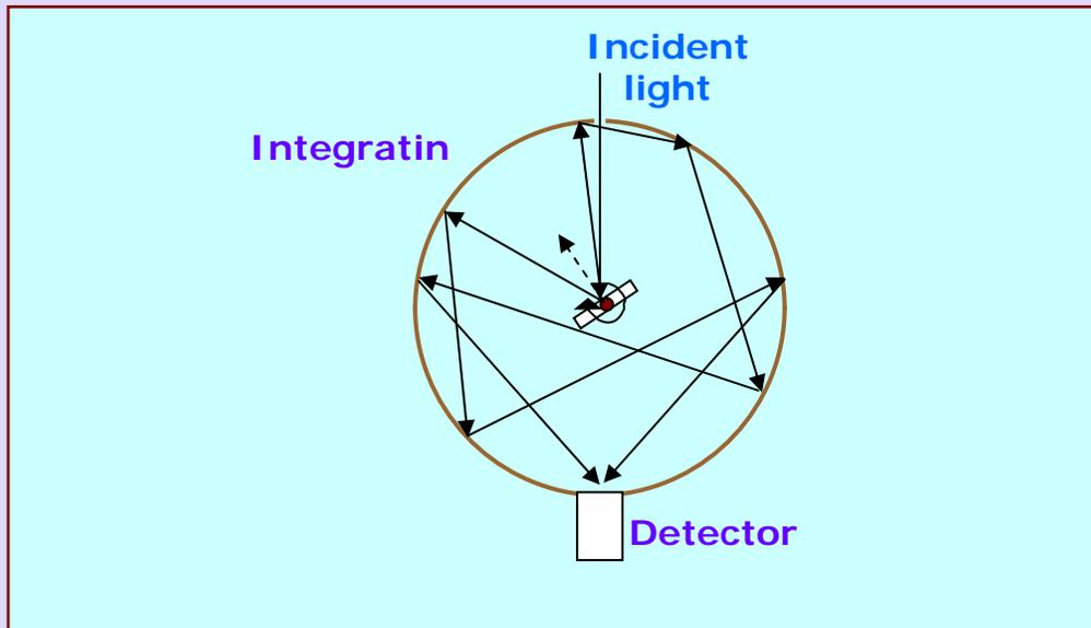
**Figure 30 Integrating sphere arranged for measurement of directional hemispherical reflectivity**
