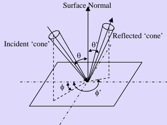
**Figure 23 Biangular reflection at a surface**
