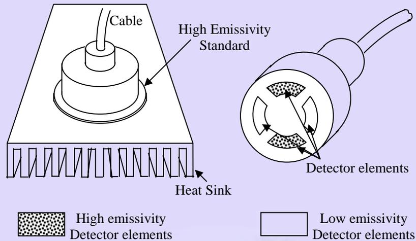
**Figure 33 Schematic of the portable emissometer**
