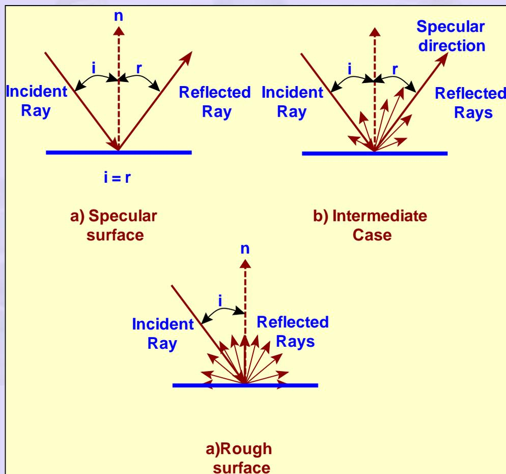
Figure 22 Schematic representation of reflection at an opaque surface
