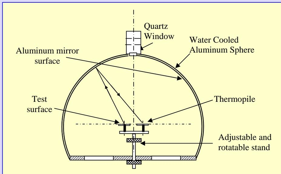
**Figure 31 Integrating radiometer**
