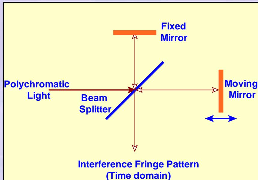
Figure 26 Schematic of a Fourier Transform Infrared Spectrometer
