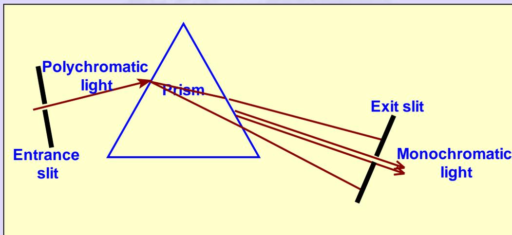
Figure 24 Schematic of a Prism Monochromator
