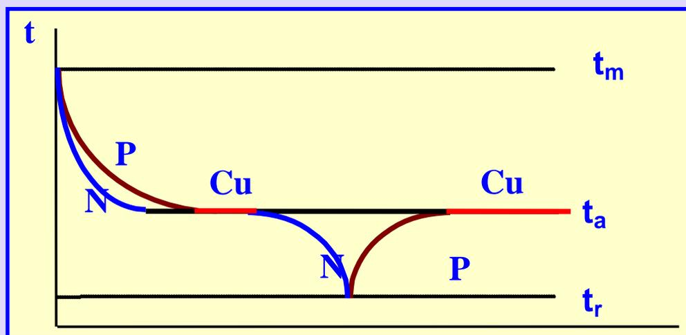
**Figure 13 Temperature variations along the wires**
