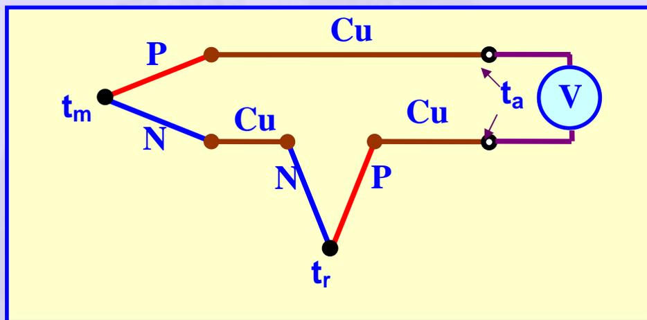
Figure 10 Practical thermocouple circuit
