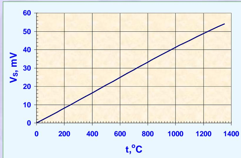
Figure 16 Seebeck volts – temperature relationship for K type thermocouple
