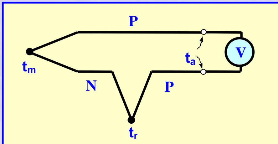
**Figure 8 Simple thermocouple circuit**
