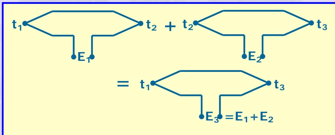
**Figure 12 Explanation of the law of intermediate temperatures**
