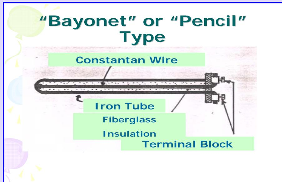
**Figure 19 Bayonet or pencil type of thermocouple probe**
