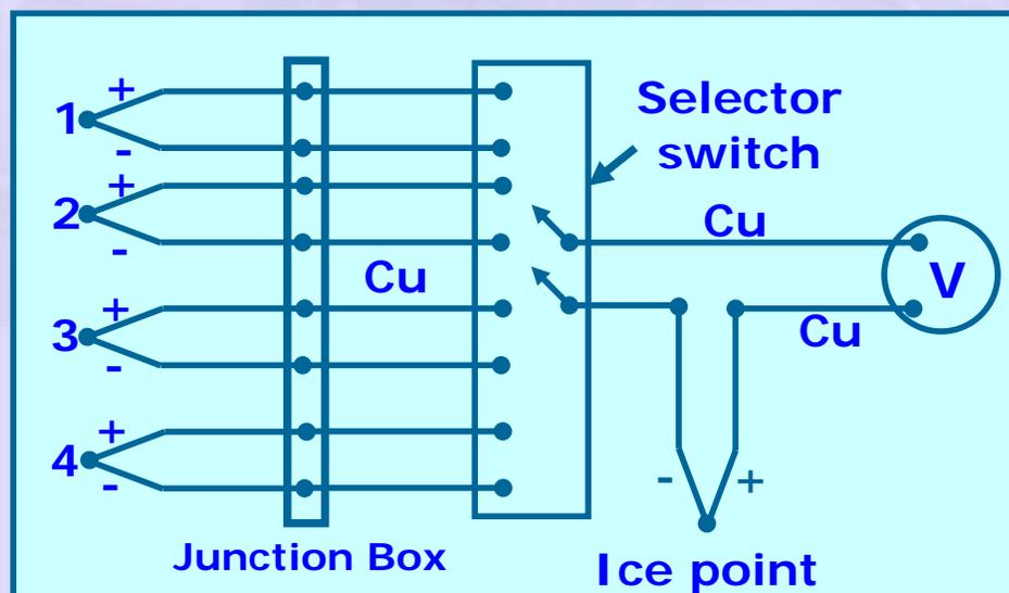
**Figure 15 Many measuring junctions with a single reference junction**
