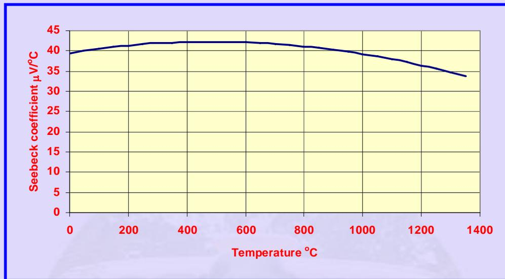
**Figure 7 Variation of Seebeck coefficient with temperature for K type thermocouple**
