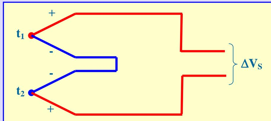
**Figure 20 Differential thermocouple for the direct measurement of temperature difference**
