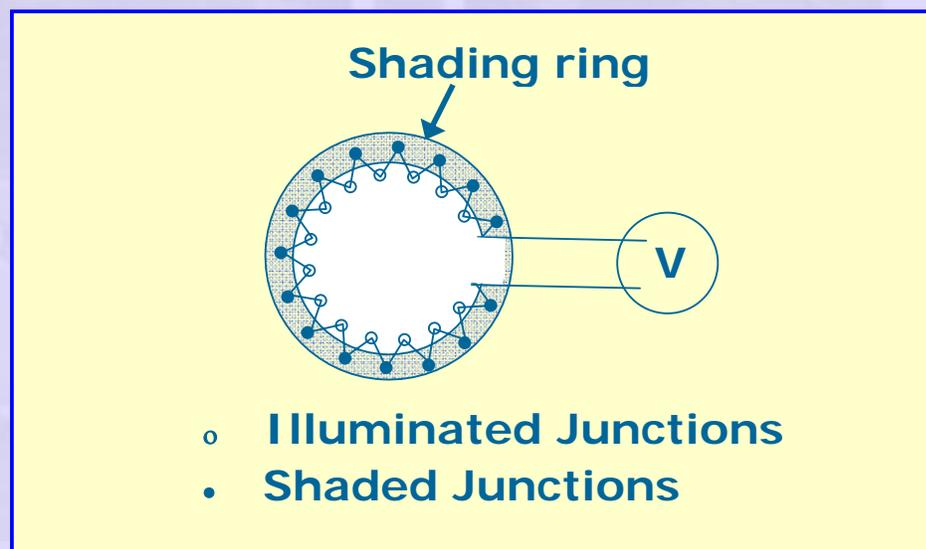
Figure 21 Several differential thermocouples in series forming a thermopile
