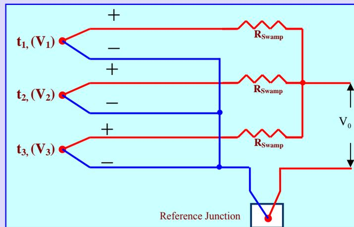
**Figure 23 Thermocouples connected in parallel and with “Swamp” resistances**
