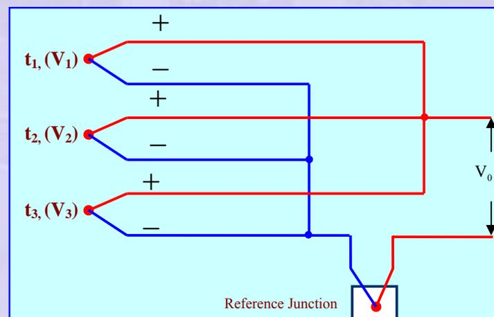
**Figure 22 Thermocouples connected in parallel**
