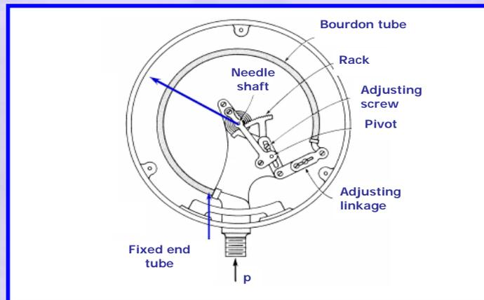
**Figure 68 Schematic of a Bourdon pressure gage**
