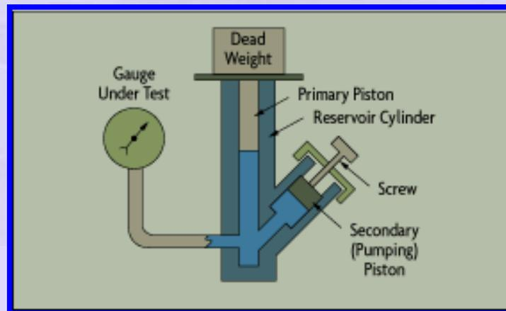
Figure 70 Schematic of a dead weight tester
