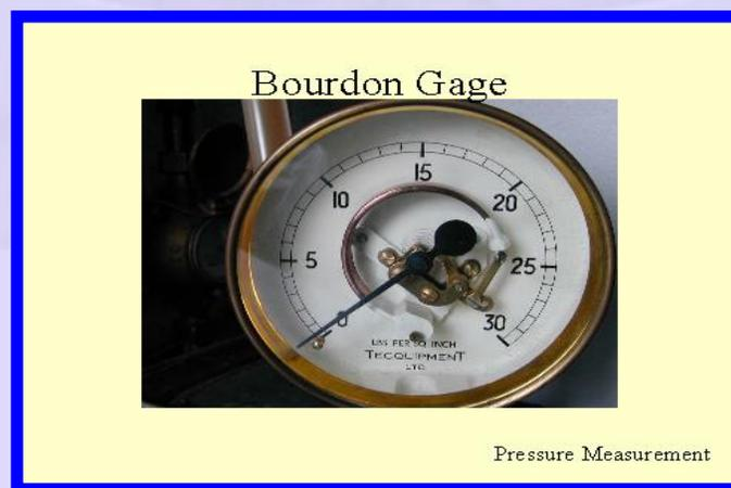
**Figure 69 Photograph of a Bourdon gage taken from the web**
