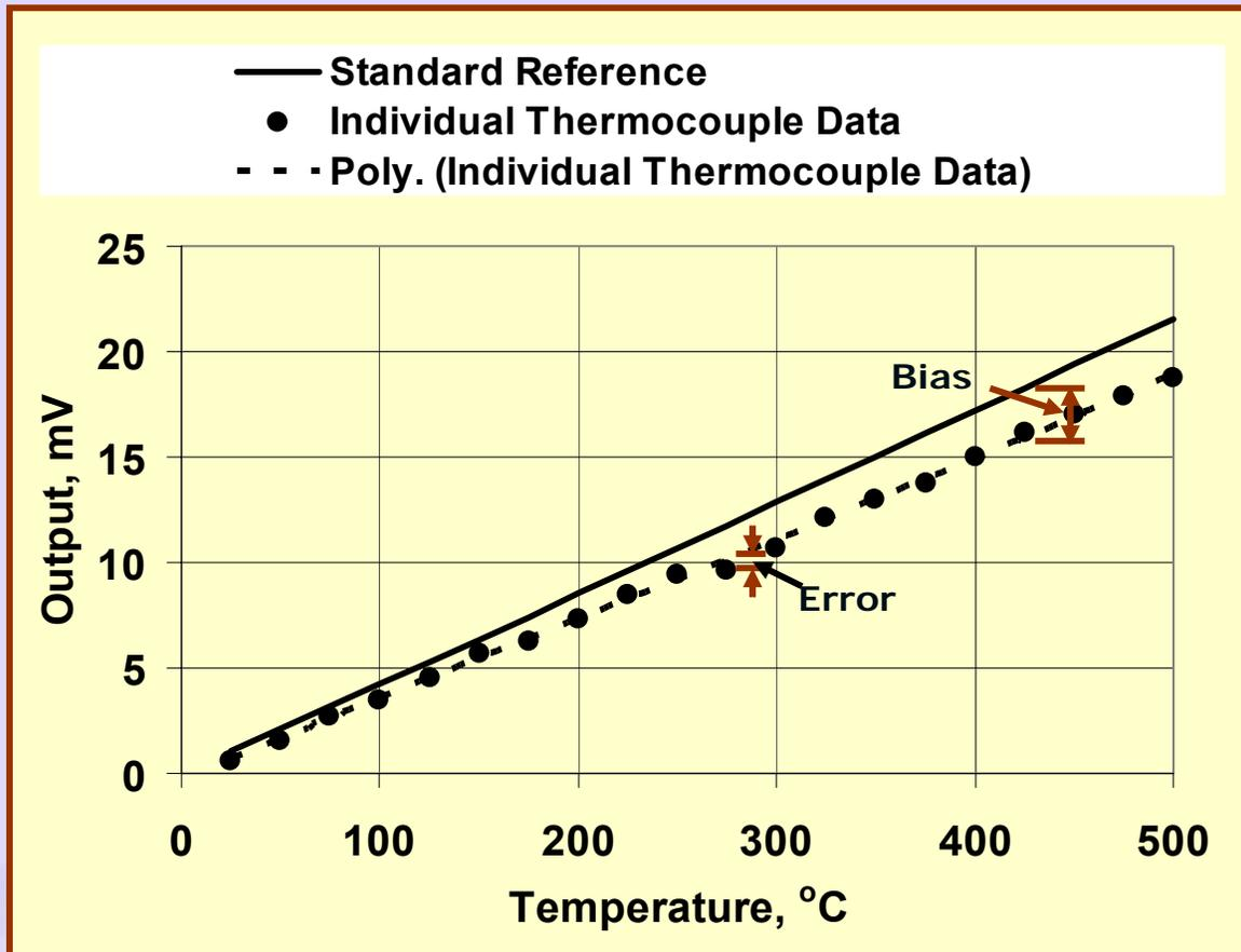
**Figure 4 Example showing the presence of systematic and random errors in data.**
