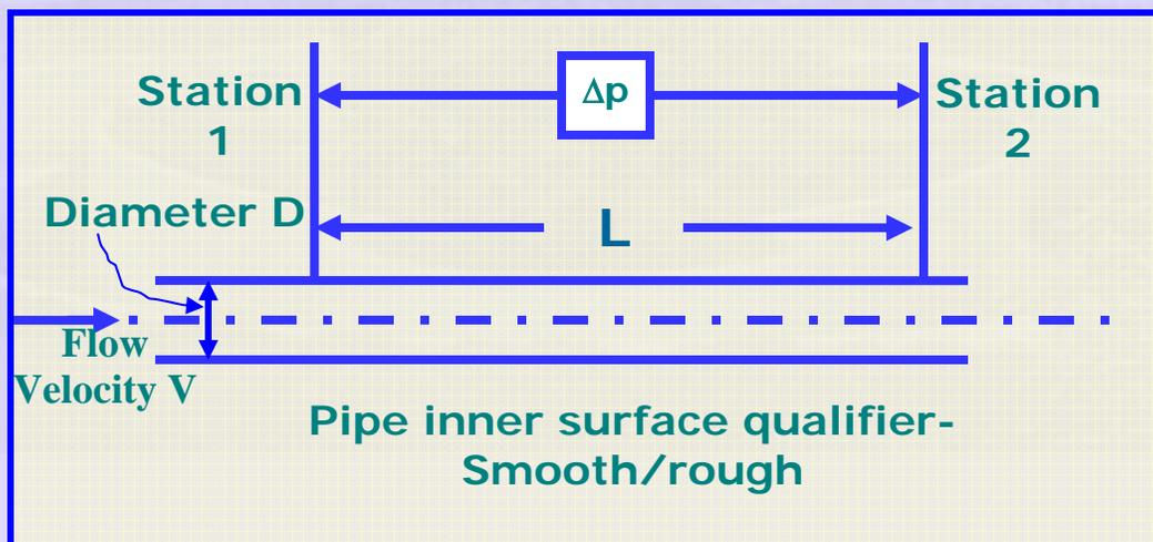
Figure 16 Schematic of an experimental set up for friction factor measurement in pipe flow
