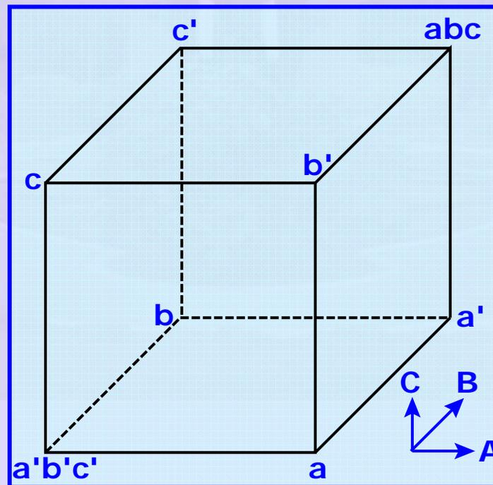
Figure 15 Three factors system with two levels. All possible values are given by the corners of the cube.
