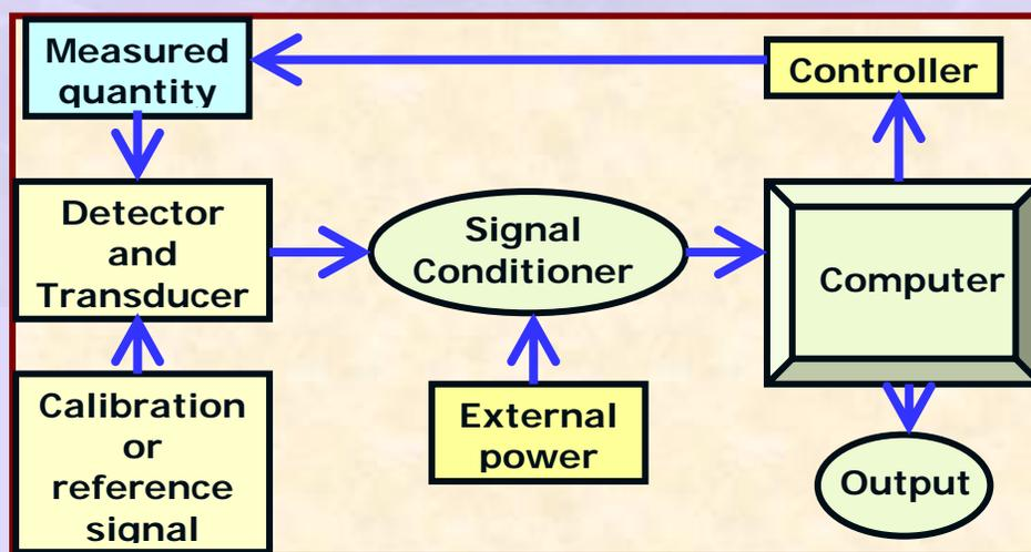
**Figure 2 Schematic of a general measurement system**
