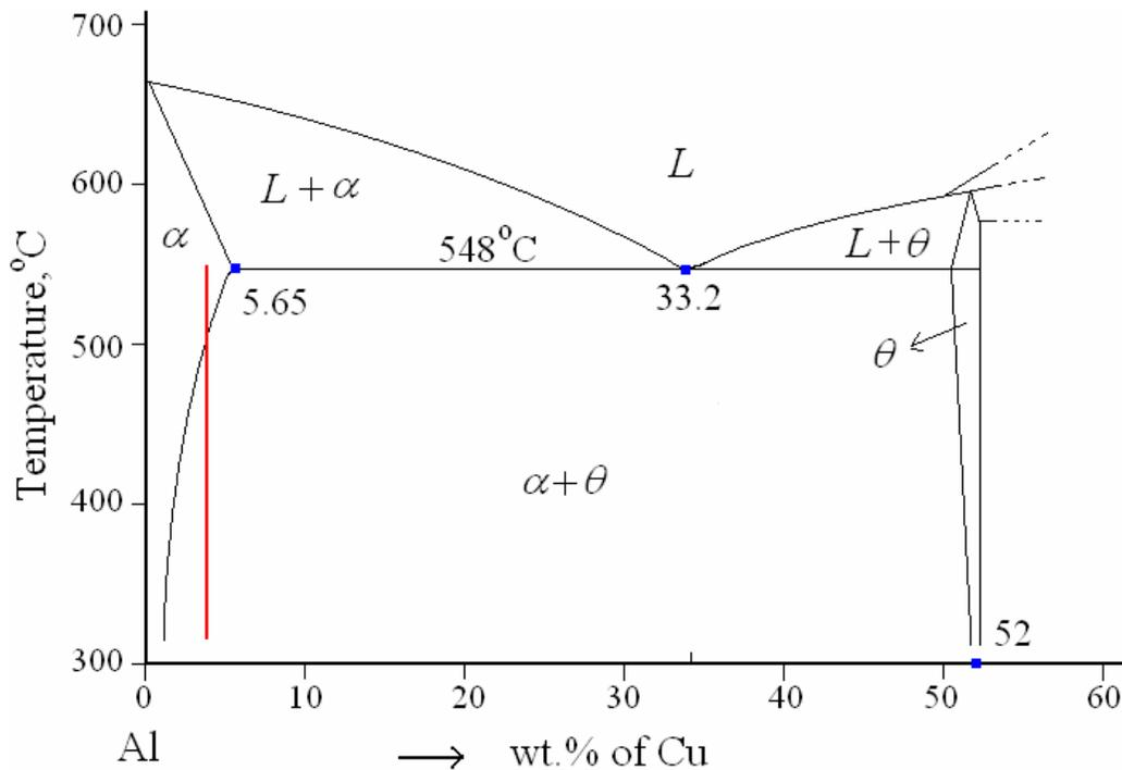
**Figure-10:** Aluminium rich end of Al-Cu phase diagram.
