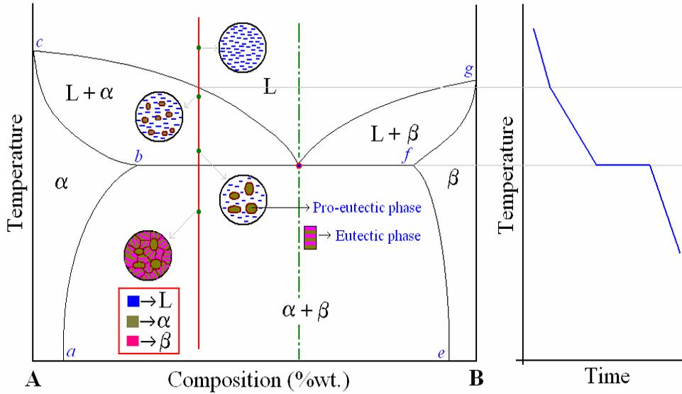
**Figure-6:** Cooling curve and micro-structure development for eutectic alloy that passes through hypo-eutectic region.
