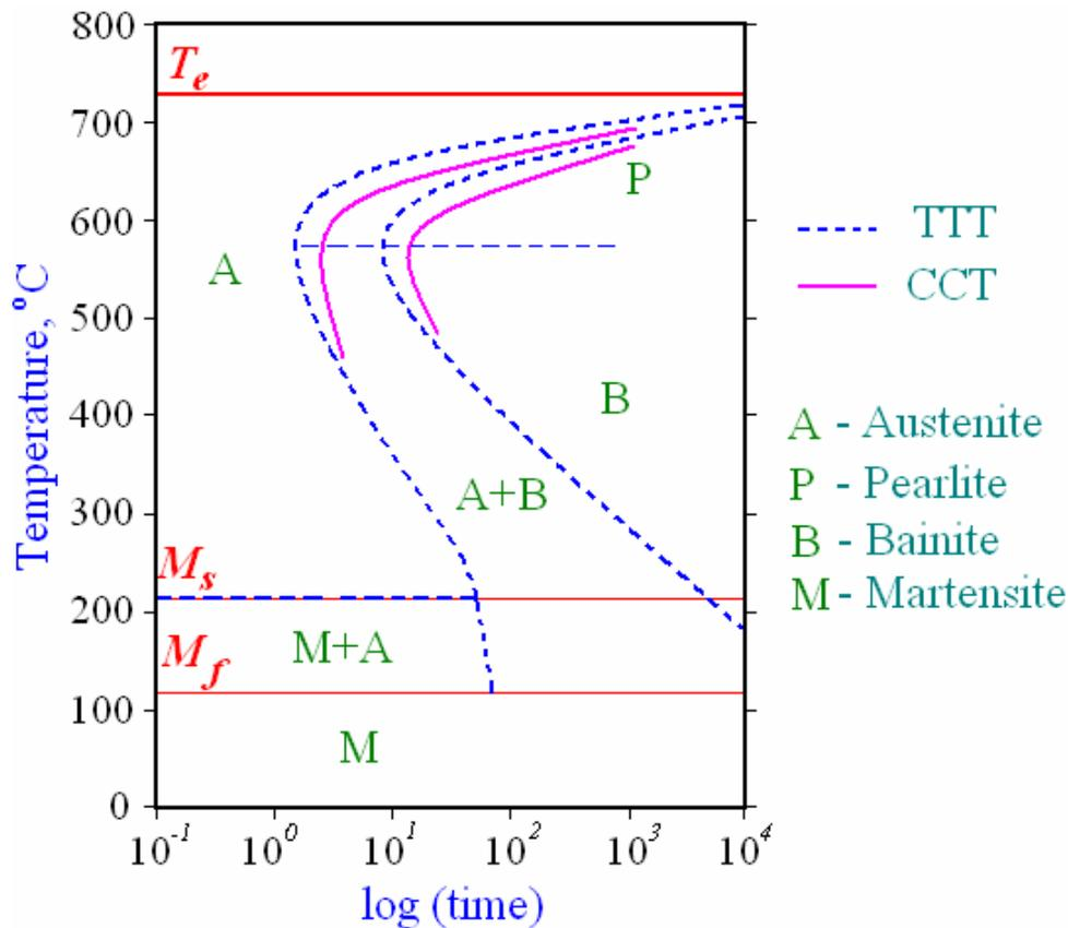
**Figure-13:** Superimposition of TTT and CCT diagrams for a eutectoid steel.
