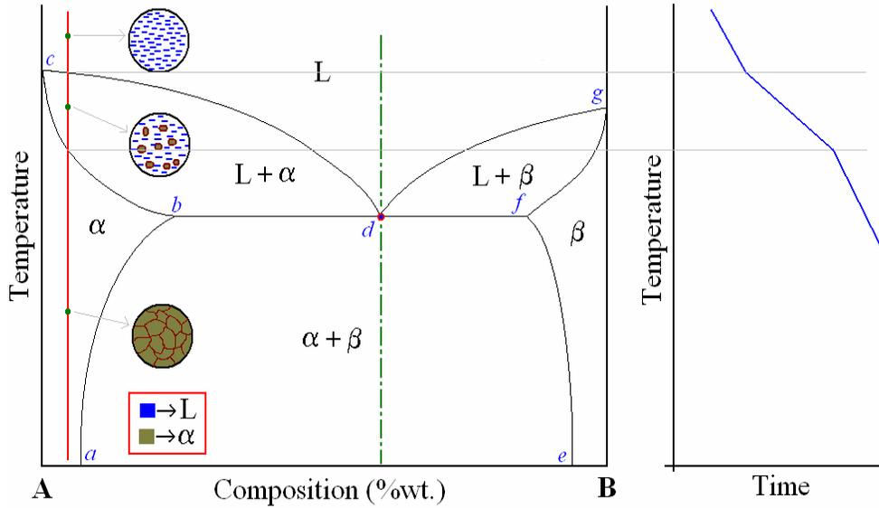
**Figure-4:** Cooling curve and micro-structure development for eutectic alloy that passes mainly through terminal solid solution.
