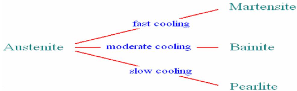
**Figure-12:** Transformations involving austenite for Fe-C system
