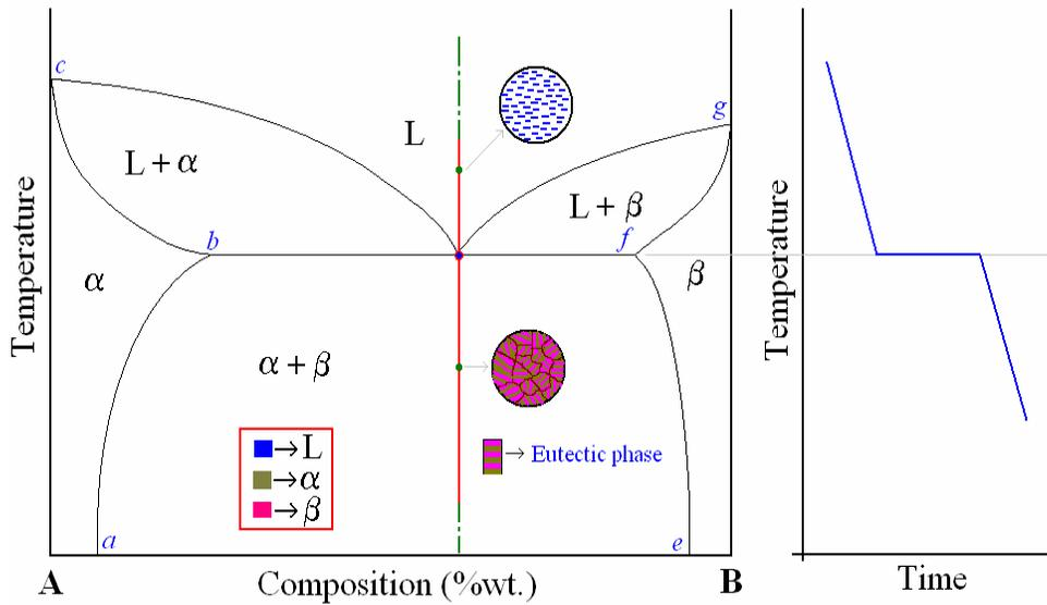
**Figure-7:** Cooling curve and micro-structure development for eutectic alloy that passes through eutectic-point.
