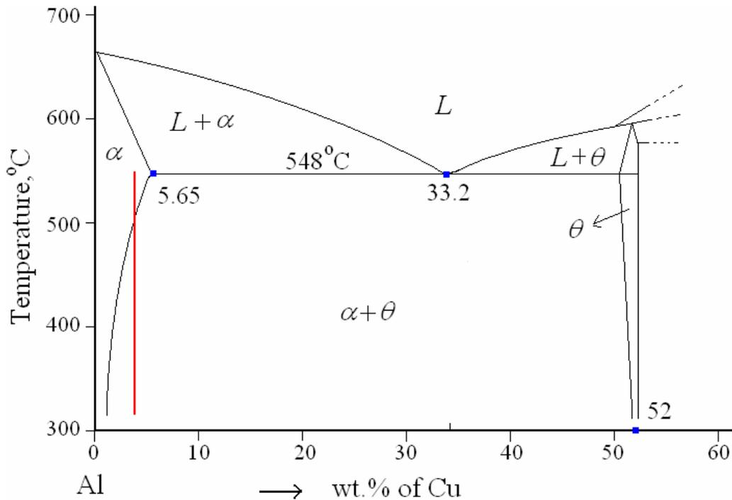
**Figure-8:** Aluminium rich end of Al-Cu phase diagram.
