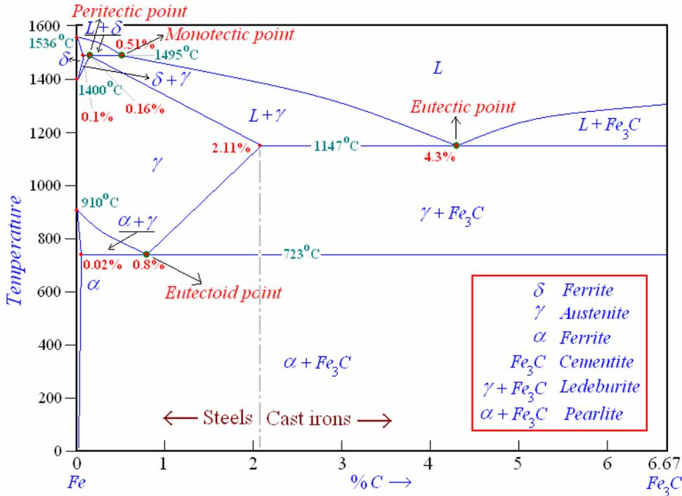
**Figure-10:** Iron – Iron carbide phase diagram.
