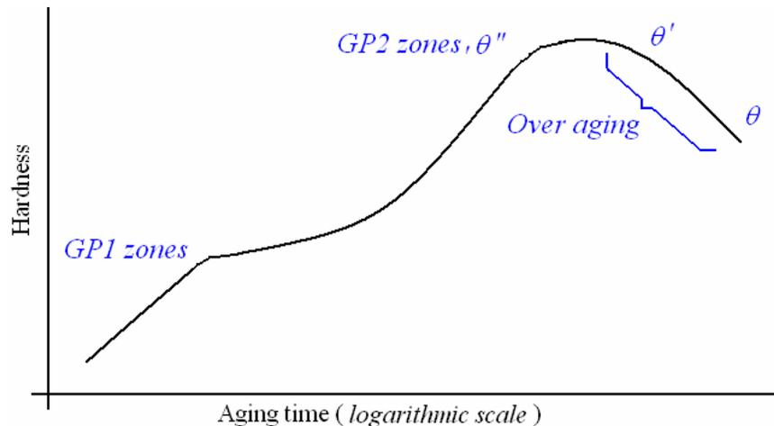
**Figure-9:** Correlation of structures and hardness for Al-4%Cu alloy.
