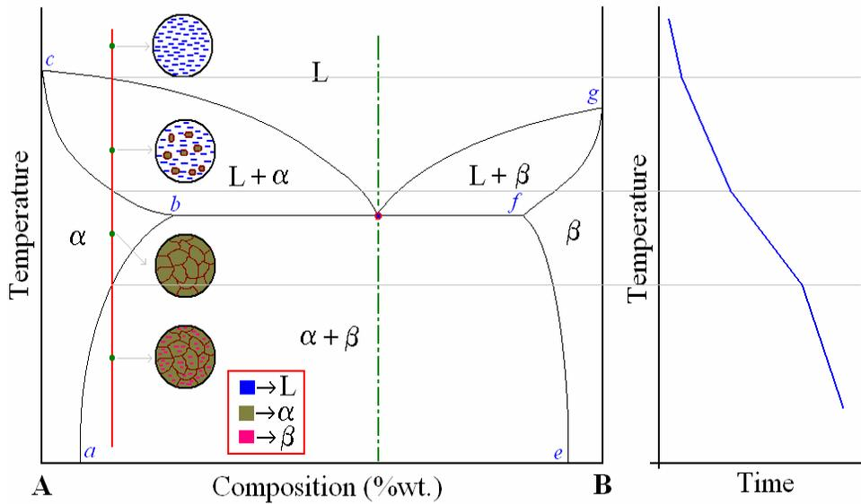
**Figure-5:** Cooling curve and micro-structure development for eutectic alloy that passes through terminal solid solution without formation of eutectic solid.
