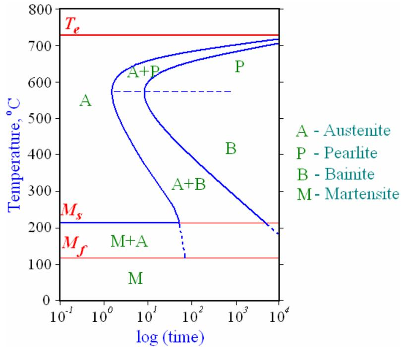
**Figure-11:** TTT diagram for eutectoid steel.
