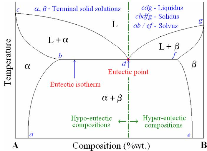
**Figure-3:** Typical phase diagram for a binary eutectic system.
