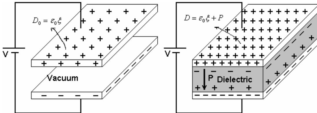
**Figure 14-5:** Schematic representation of capacitor and polarization phenomenon.
