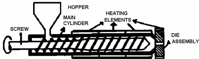
Figure 10.4: Schematic diagram of Injection molding
