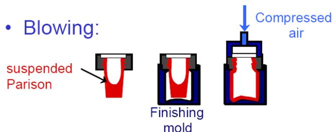
**Figure 10.1:** Schematic diagram of pressing and blowing processes
