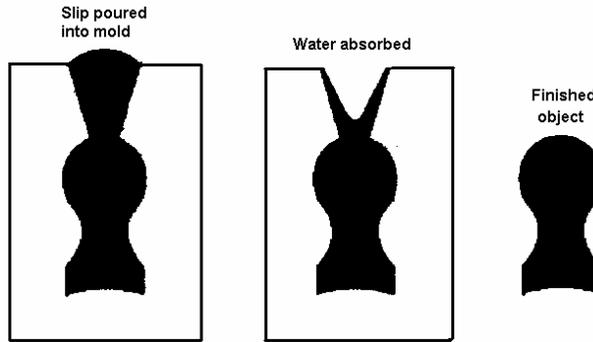
Figure 10.3: Schematic diagram of slip casting process
