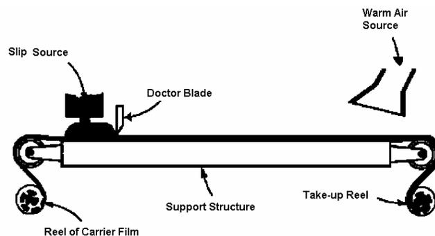
**Figure 10.2:** *Schematic diagram of tape casting process*
