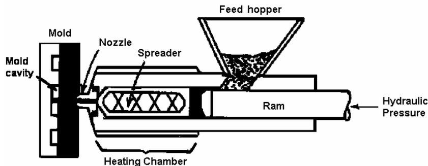
*Figure 10.5: Schematic diagram of Injection molding*
