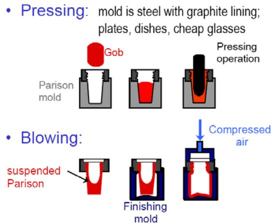
**Figure 10.1:** Schematic diagram of pressing and blowing processes
