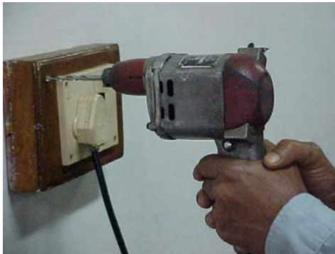
Fig. 4.2.5 Hand drill in operation
