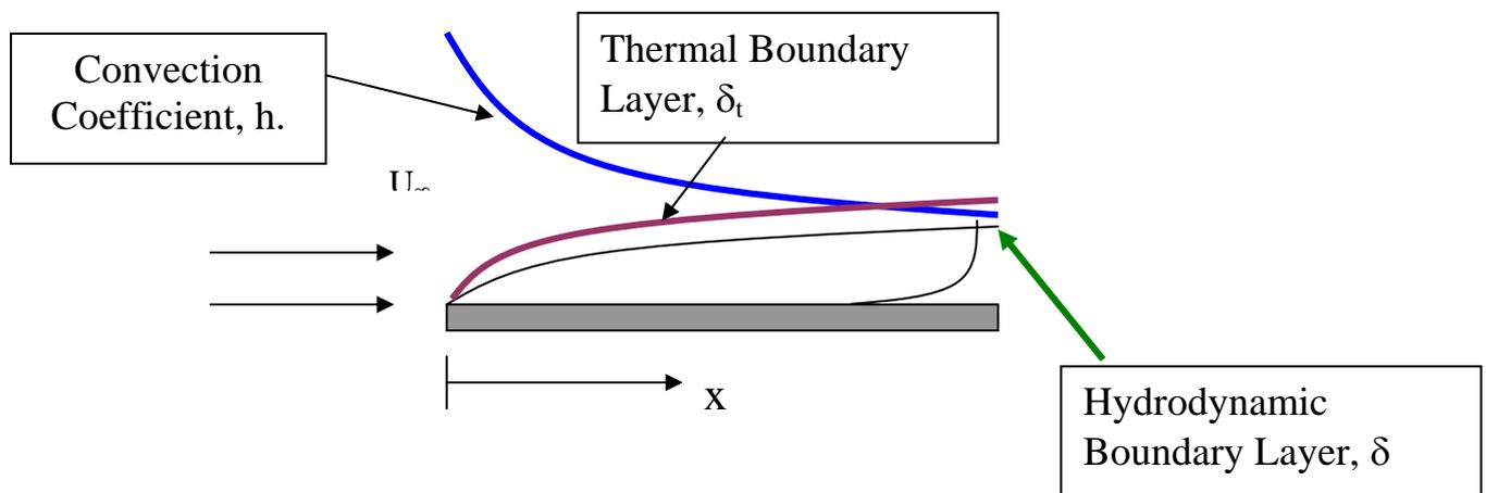
We see that as the boundary layer thickens, the convection coefficient decreases. Some designers will introduce a series of “trip wires”, i.e. devices to disrupt the boundary layer, so that the buildup of the insulating layer must begin anew. This will result in regular “thinning” of the boundary layer so that the convection coefficient will remain high.
