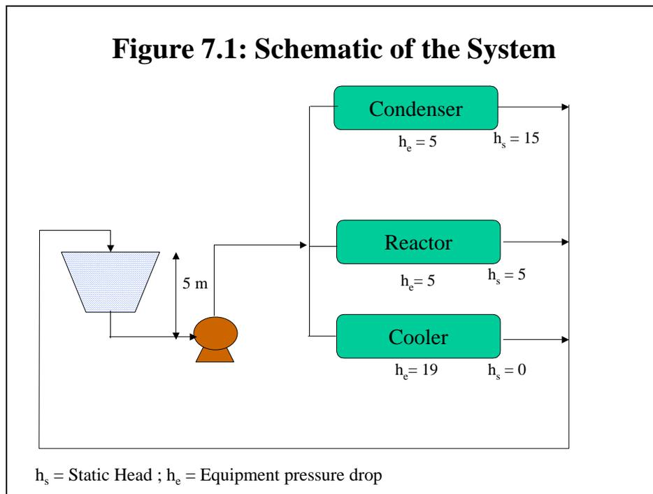
The step-by-step approach for determining system resistance curve is given below.
