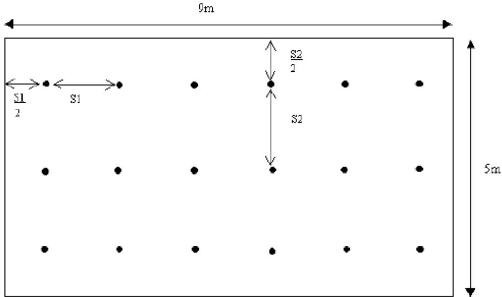
Therefore in this example the spacing between points along rows along the length of the interior =  $9 \div 6 = 1.5\text{m}$  and the distance of the 'end' points from the wall =  $1.5 \div 2 = 0.75\text{m}$ .
