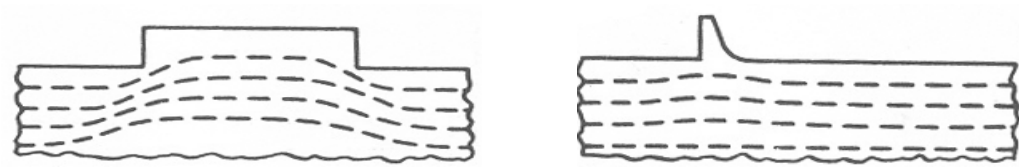
(c) Force flow around a wide projection Force flow around a narrow projection: Low stress concentration.
