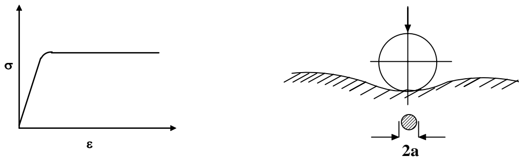
1.2.6.1F- Stress-strain diagram of an elastic-perfectly plastic material and the plastic indentation.
