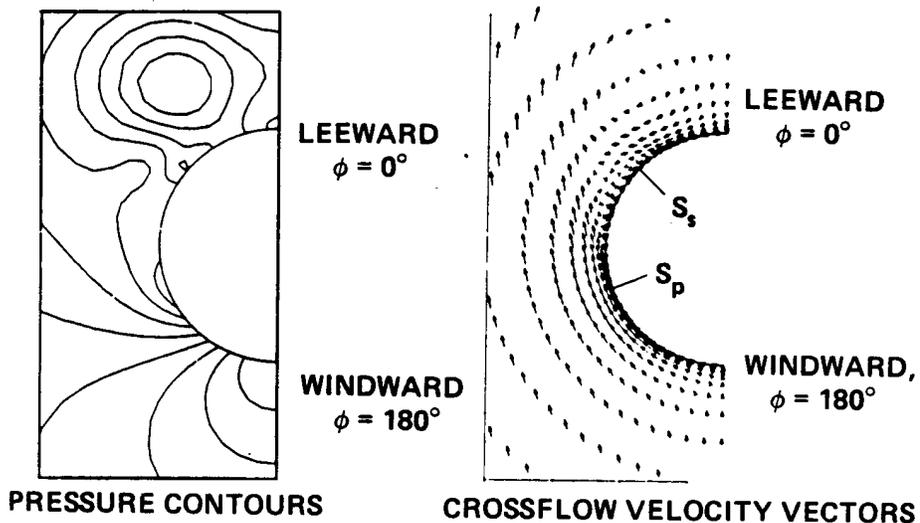
FIGURE 32. Hemisphere-Cylinder at  $M_\infty = 1.2, \alpha = 19^\circ$ .
