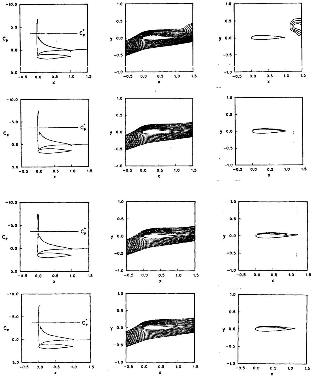
FIGURE 29. Unsteady Solution at  $M_\infty = 0.4$ ,  $\alpha = 15^\circ$ .
