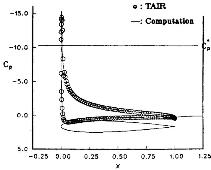
FIGURE 27. Inviscid Solution Compared with TAIR Result.
