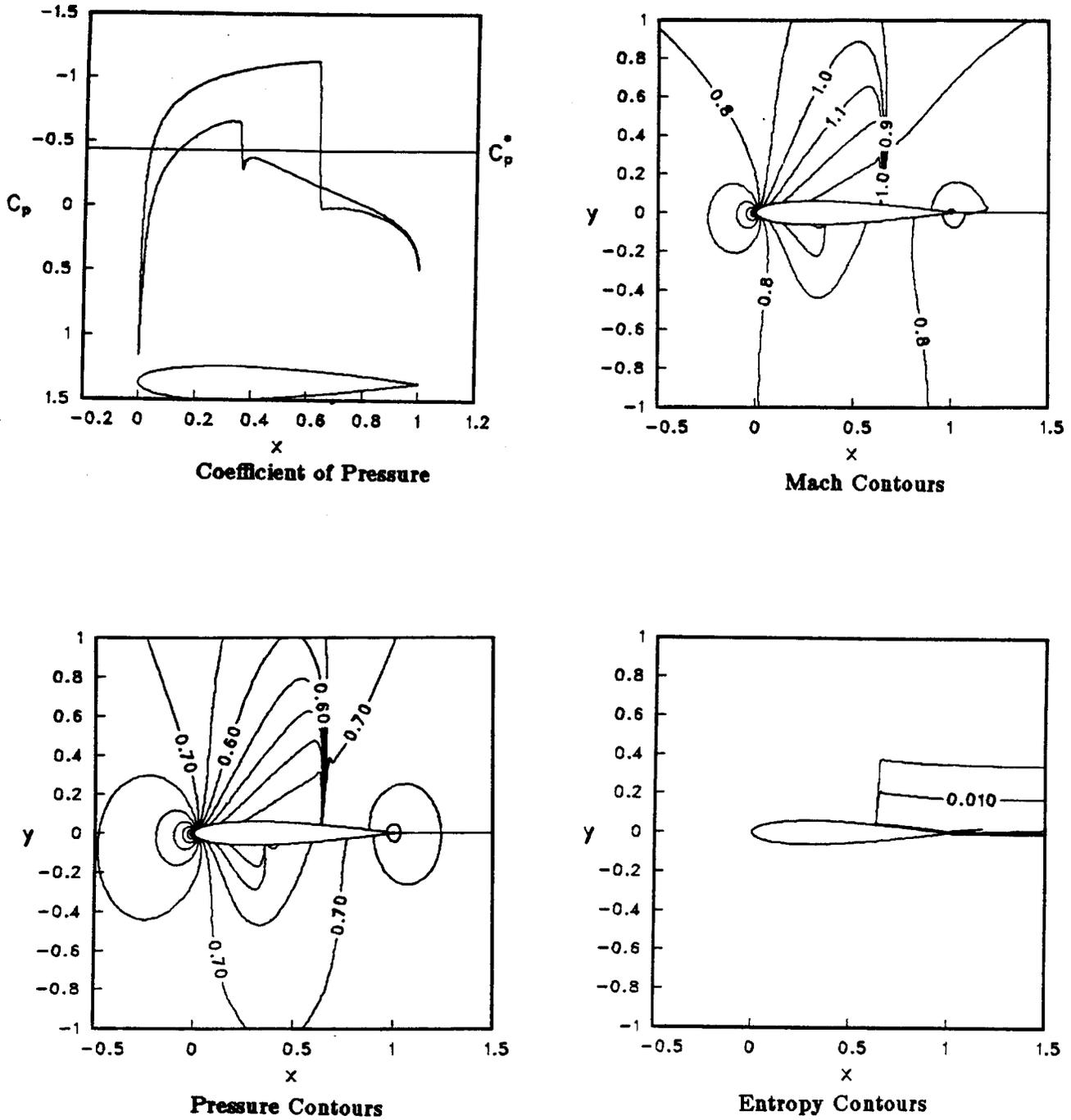
FIGURE 19. ARC2D Results for 248 by 49 Grid.
