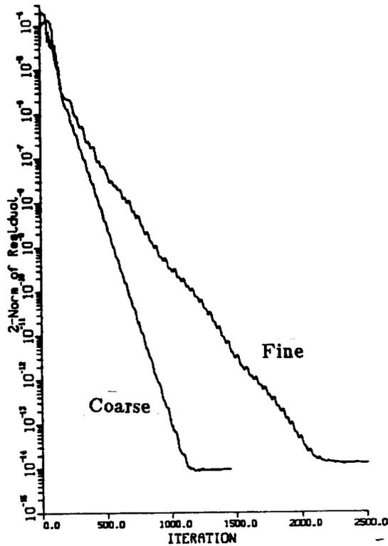
FIGURE 21. Convergence History vrs Iteration for ARC2D Results.
